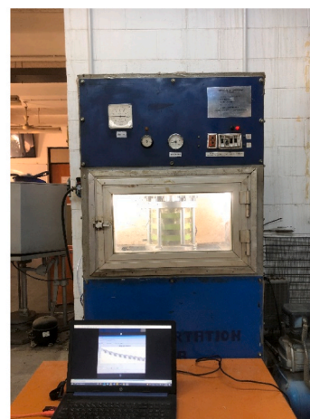
(b) Triaxial test under controlled temperature
