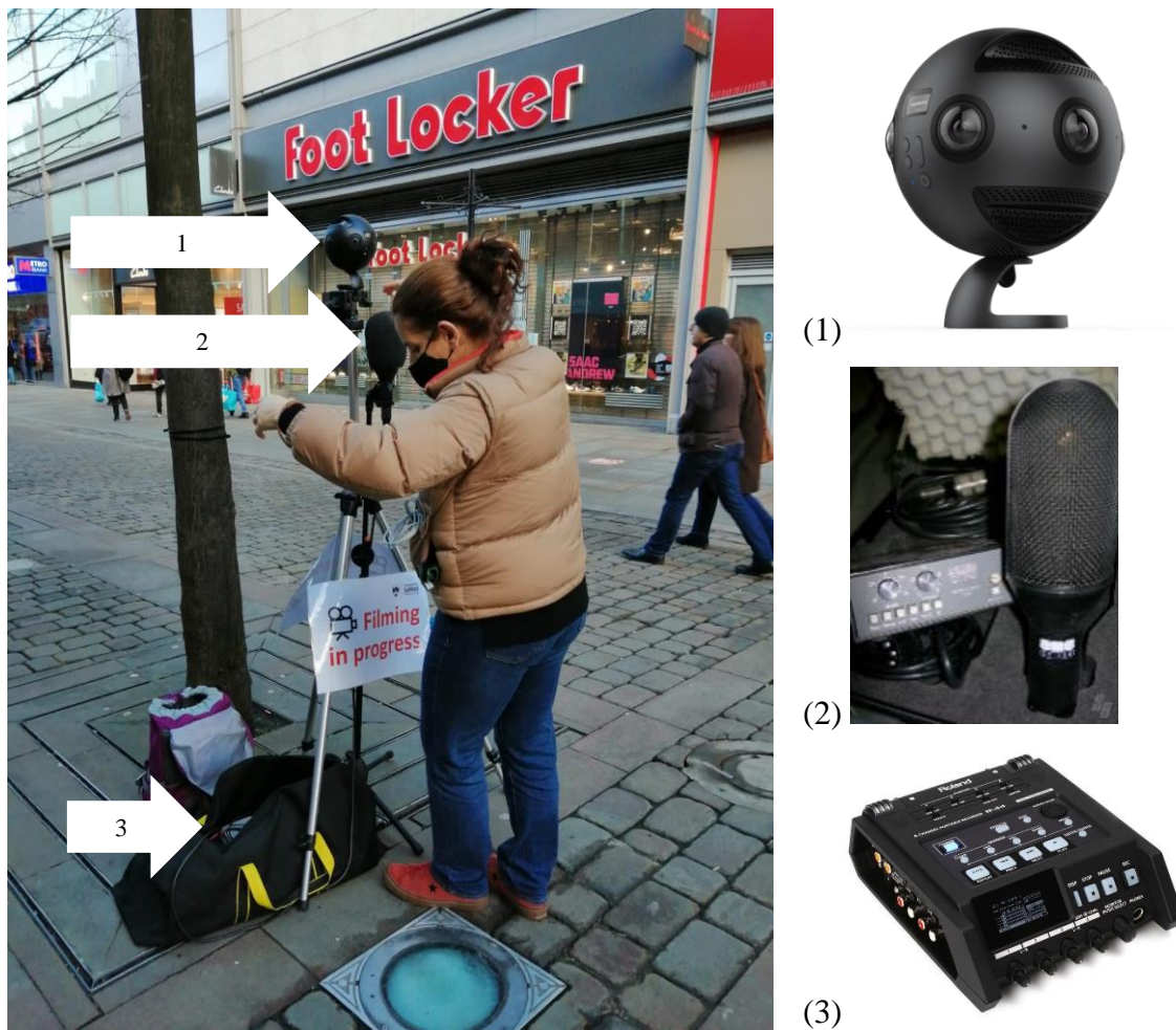
FIGURE 27: EQUIPMENT SETUP AT MARKET STREET WITH INSTA 360 PRO2 VR CAMERA (1), SOUND FIELD MICROPHONE ST250 (2), AND EDIROL R44 RECORDER (3).
