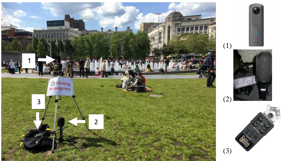
FIGURE 21: EQUIPMENT SETUP AT PICCADILLY GARDENS WITH RICOH THETA CAMERA (1), SOUND FIELD MICROPHONE ST250 (2), AND ZOOM H6 HANDY RECORDER (3).
