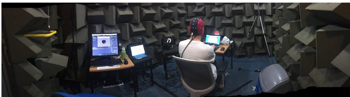
FIGURE 28: EQUIPMENT ARRANGEMENT IN THE SEMI-ANECHOIC CHAMBER FOR EXPERIMENT.
