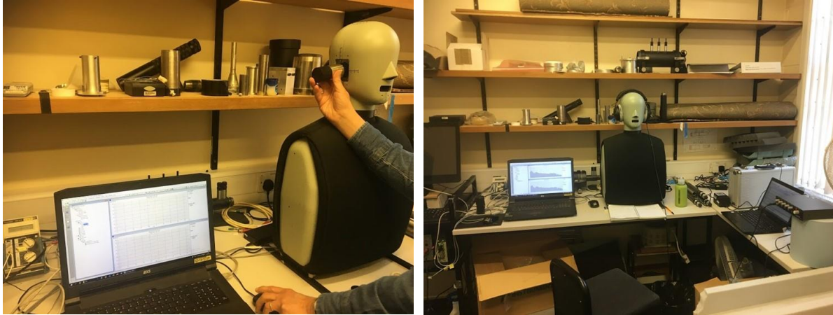
FIGURE 25: HATS INTERNAL MICROPHONE CALIBRATION ON THE LEFT, AND SETUP FOR SAMPLE CALIBRATION ON THE RIGHT.
