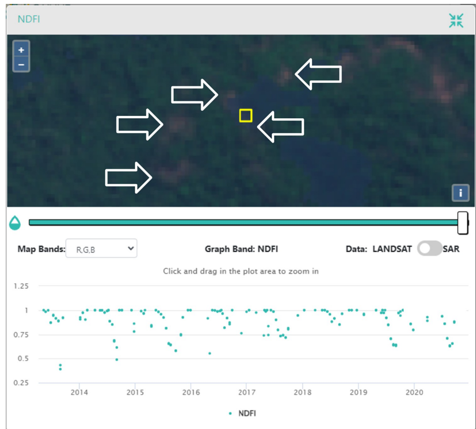
Fig 12. Plot in the CEO disturbances validation project. This pixel was misclassified as Degradation. NDFI time series show a seasonal pattern with lower NDFI values around August of each year. It is important to note that the MapBiomas classification maps these areas as “Savannic Forest Formations”. Basemap imagery is from Sentinel-2 (European Space Agency).
