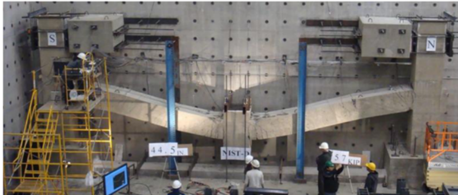
Figure 19: Full-scale seismic detailed sub-assembly for column-removal testing [160]
