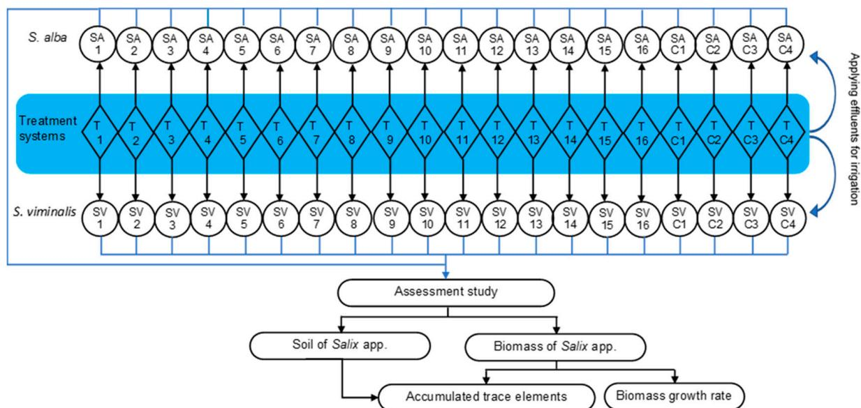
**Figure 2.** Schematic drawing of the experimental design and the flow directions within the system.
