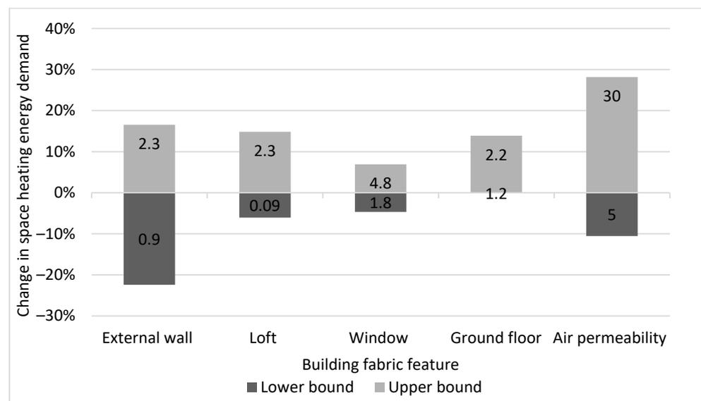
**Figure 6.** Percentage change relative to the base case for combined lower and upper bounds for five building fabric features, with the data labels showing the input parameters (U-values and air permeability) in Table 3.
