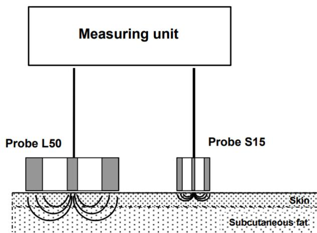
Figure 24. Schematic illustration of the dielectric measurement and induced electrical field in skin and SSF. Image provided by Delfin Technologies.
