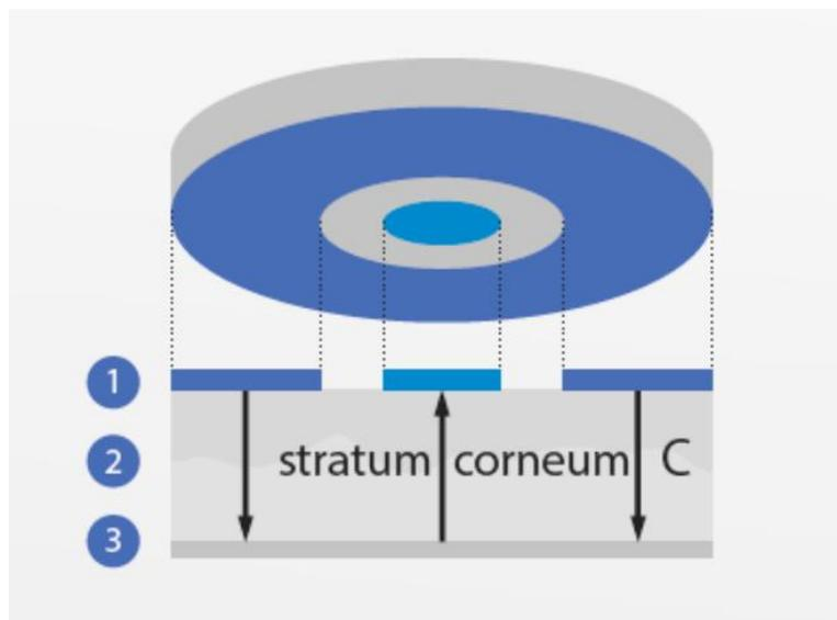
Figure 23. Demonstration of the probe head of the MoistureMeter SC™. Image extracted from [https://delfintech.com/products/moisturemetersc/?gclid=EAlaIQobChMlo7aQm-qP\\_gIVh-vtCh102gUEEAYASAAEgIDpfd\\_BwE](https://delfintech.com/products/moisturemetersc/?gclid=EAlaIQobChMlo7aQm-qP_gIVh-vtCh102gUEEAYASAAEgIDpfd_BwE) on 24/02/23.
