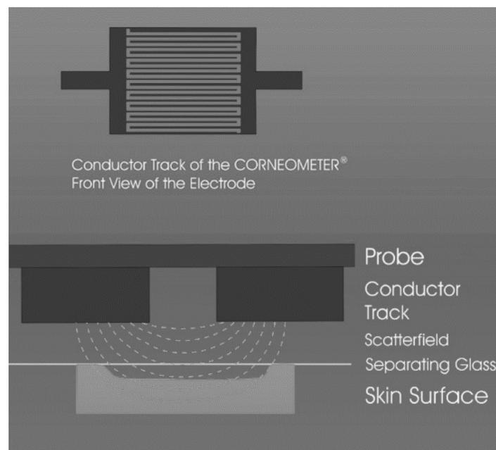
Figure 22. Diagram demonstrating the probe structure and signal penetration of the Corneometer® CM825, extracted from [http://www.dproscientific.com/assets/brochure\\_cm825.pdf](http://www.dproscientific.com/assets/brochure_cm825.pdf) on 04/04/23.
