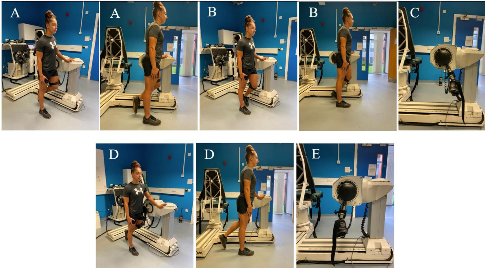
**Figure 4.1** Images of Kin Com testing set up. **(A)** Hip extension, with attachment cuff above the knee; **(B)** Combined hip extension and knee extension with attachment cuff below the knee; **(C)** Angle set up of dynamometer lever arm for hip extension and combined hip and knee extension; **(D)** Hip flexion with attachment cuff above the knee; **(E)** Angle set up of dynamometer lever arm for hip flexion *Note: Images show left leg, the same was replicated for the right leg*
