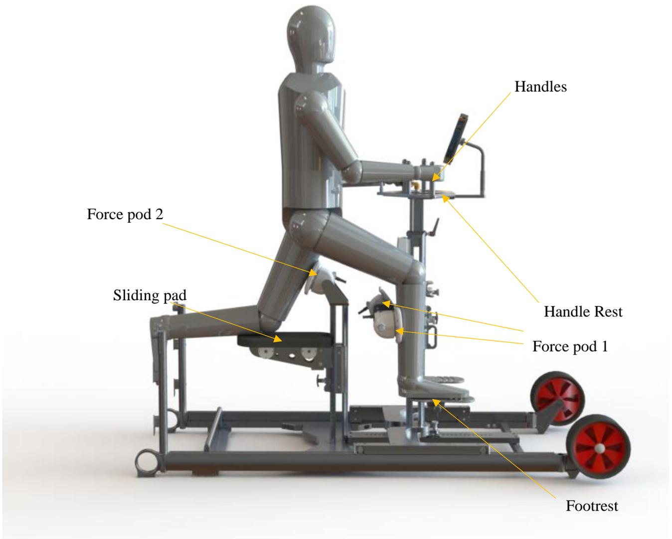
**Figure 4.0** Biostrain device and subject set up
