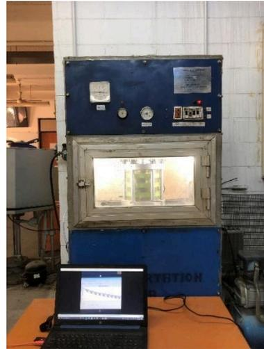
(b) Triaxial test under controlled temperature
