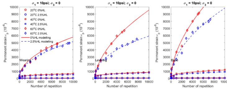
Figure 4. The represented permanent deformation by the 1<sup>st</sup> term of the Francken model.
