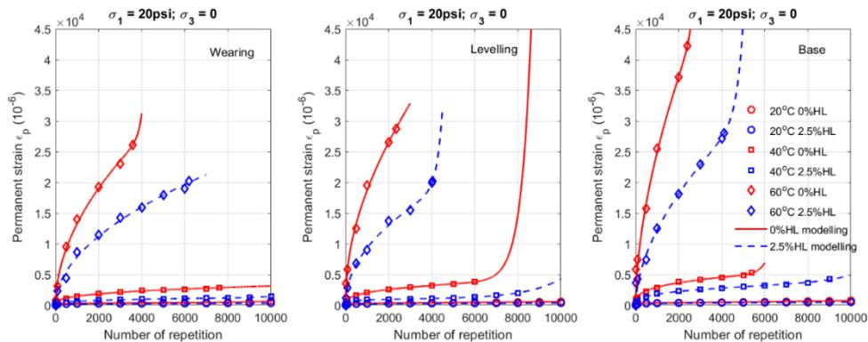
(b) Axial stress ( $\sigma_1$ ) is 20 psi (137.9 kPa), confining stress ( $\sigma_3$ ) is 0
