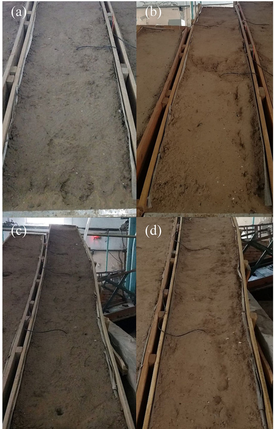
FIGURE 11 Observed splash erosion under different conditions. ((a) 3-m slope length and 60 mm/h rainfall intensity; (b) 3-m slope length and 100 mm/h rainfall intensity; (c) 5-m slope length and 60 mm/h rainfall intensity; (d) 5-m slope length and 100 mm/h rainfall intensity).
