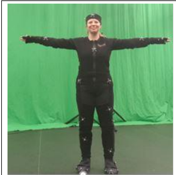
Figure 6 - Lucie in the MoCap specialised suit with markers set on the suit.
