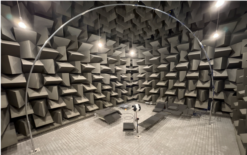
Fig. 8. Acoustic test setup of EDF in the anechoic chamber [From [36]].
