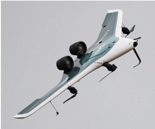
Fig. 26. Integrated propulsion module (IPM) developed for flight testing [Courtesy of Greenjets Ltd.]
