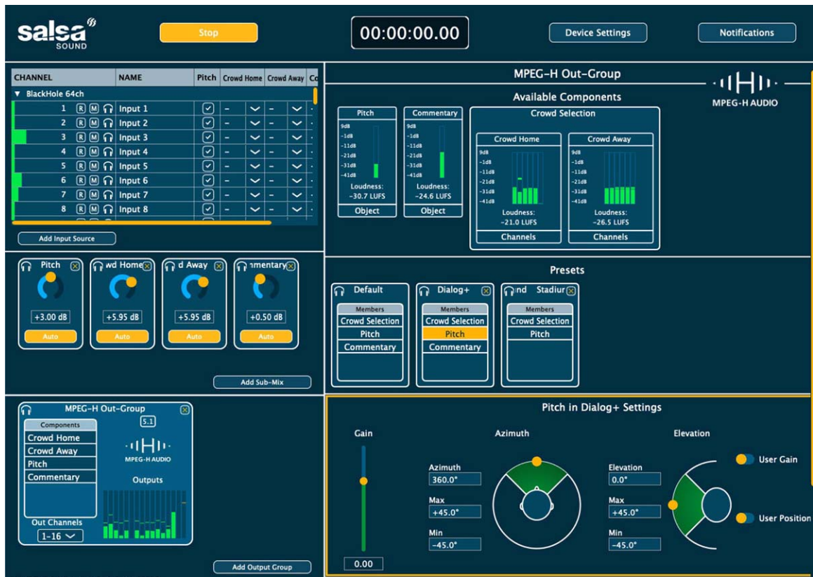
Fig. 3. MIXaiR interface with signal flow top to bottom on left panel. Right panel shows edit view of any highlighted left-panel object, in this case, the MPEG-H output group with authoring controls.
