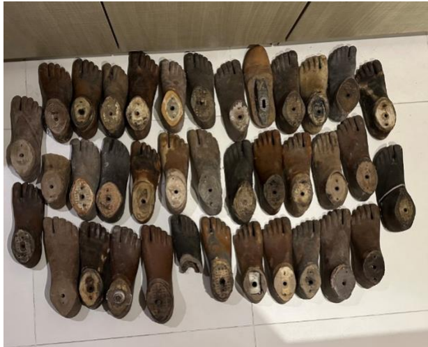
Broken prosthetic feet from SLSPO, Ragama, Sri Lanka (Photo: Dr Michael Berthaume and Dr Nicola Bailey, Kings College London)
