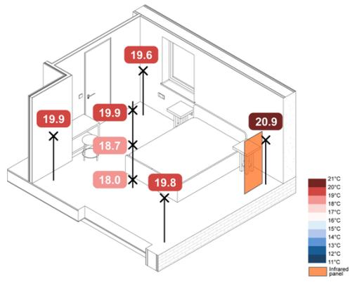
Figure 129. -5 °C Wall Mounted IR eHome2 Constant – Spatial Operative Temperatures
