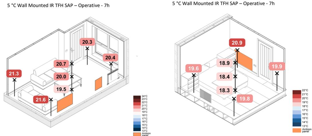
Figure 74. 5 °C Wall Mounted IR TFH SAP – Spatial Operative Temperatures
