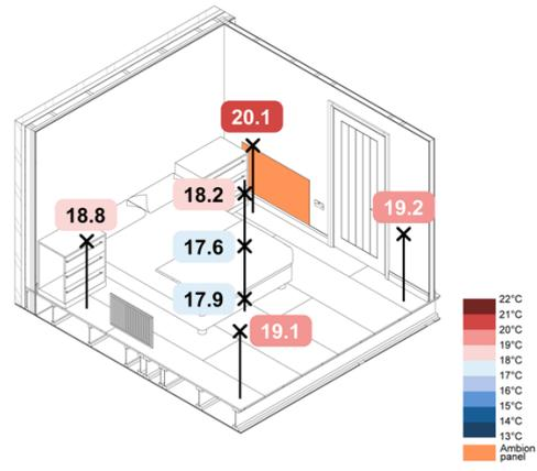
Figure 23. -5°C Wall Mounted IR TFH Constant Spatial Operative Temperatures
