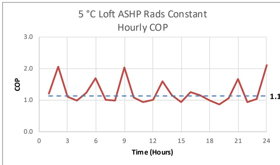
Figure 90. 5 °C Loft ASHP Rads Constant – Hourly COP
