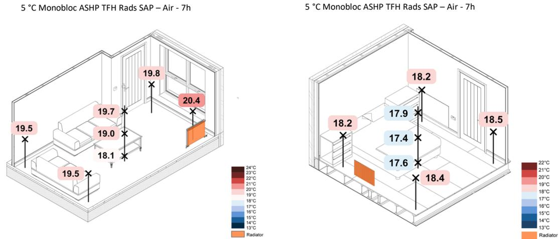
Figure 114. 5 °C Monobloc ASHP TFH Rads SAP – Spatial Air Temperatures
