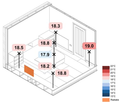
Figure 93. 5 °C Loft ASHP Rads SAP – Spatial Operative Temperatures
