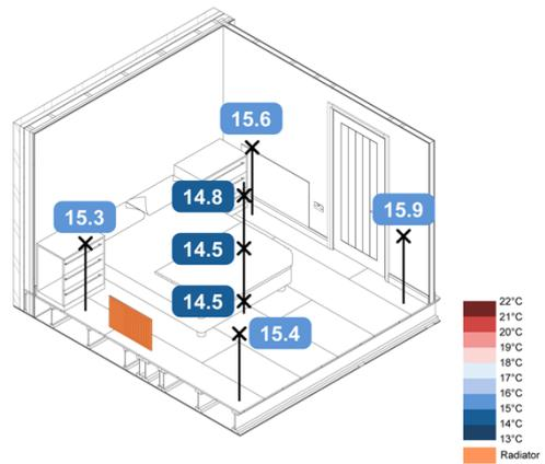
Figure 36. -5°C Loft ASHP Rads + UFH SAP – Spatial Operative Temperatures
