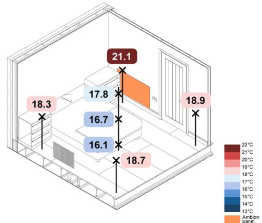
Figure 26. -5°C Wall Mounted IR TFH SAP - Spatial Air Temperatures
