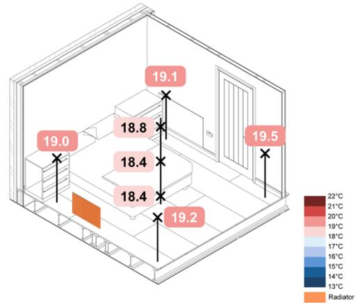
Figure 30. -5°C Loft ASHP Rads + UFH Constant - Spatial Air Temperatures
