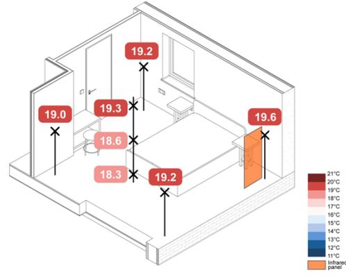
Figure 147. 5 °C Wall Mounted eHome2 Constant – Spatial Air Temperatures
