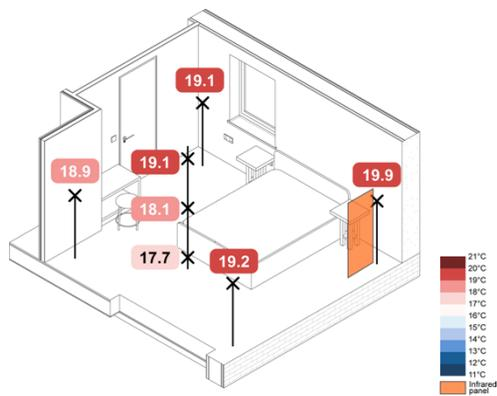
Figure 128. -5 °C Wall Mounted IR eHome2 Constant – Spatial Air Temperatures
