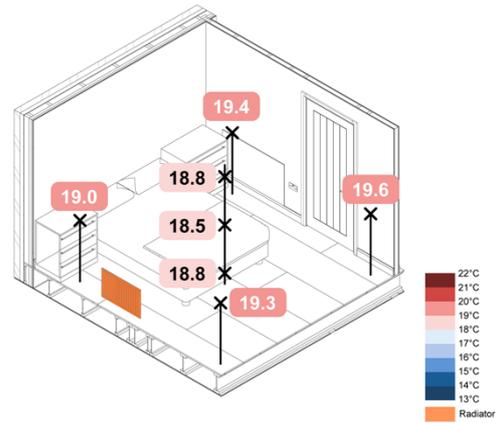
Figure 89. 5 °C Loft ASHP Rads Constant – Spatial Operative Temperatures
