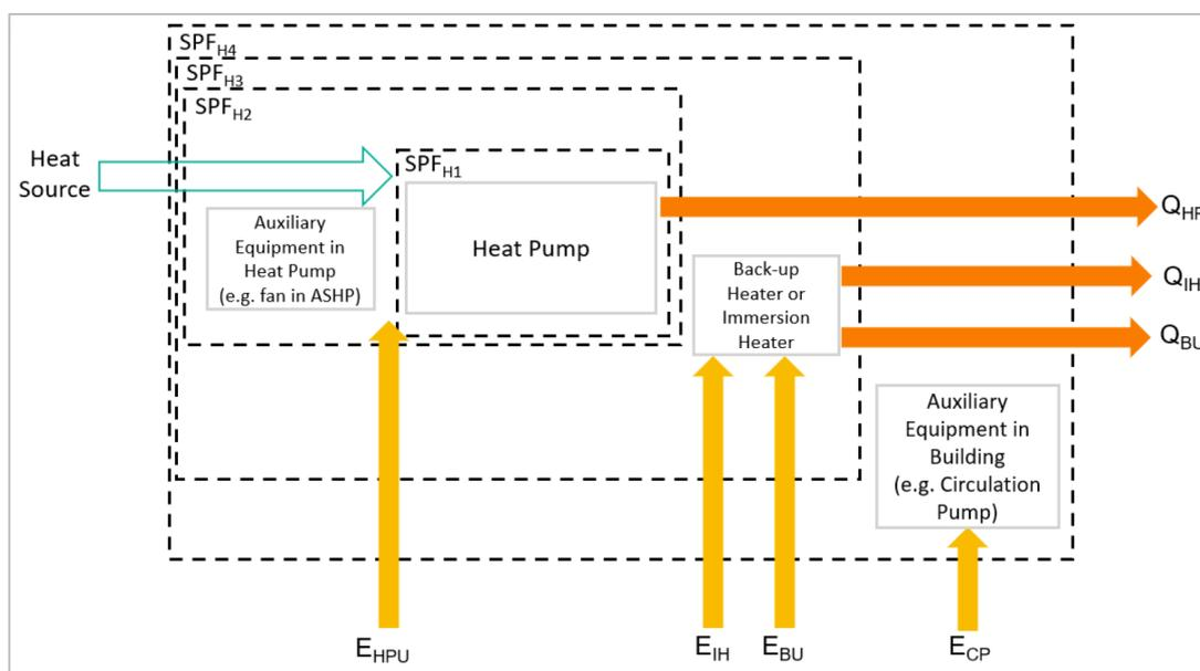
Figure 19. SPF system boundaries used to calculate coefficient of performance (COP) values. Test conditions meant that the immersion heater ( $E_{IH}$  and  $Q_{IH}$ ) was not used in the systems tests at Energy House 2.0.<sup>2</sup>
