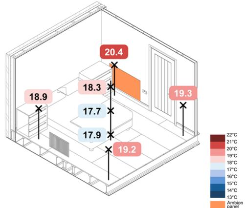
Figure 22. -5°C Wall Mounted IR TFH Constant Spatial Air Temperatures
