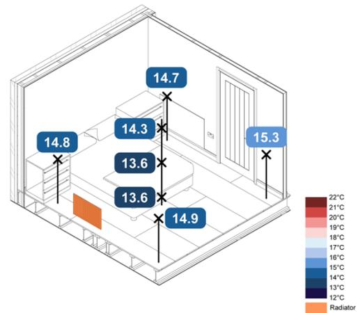
Figure 66. -5 °C Monobloc ASHP TFH Rads SAP – Spatial Air Temperatures
