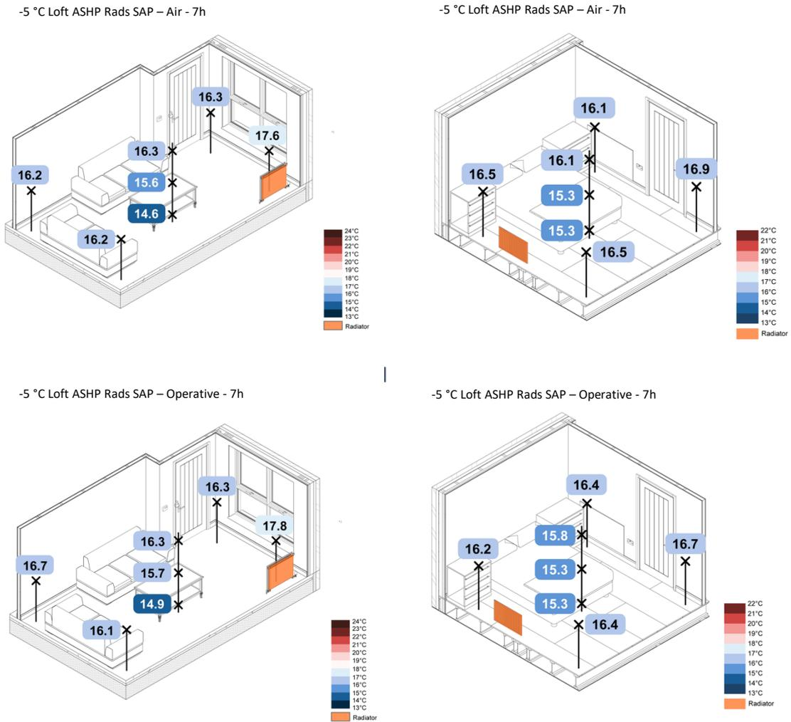
Figure 46. -5 °C Loft ASHP Rads SAP – Spatial Operative Temperatures
