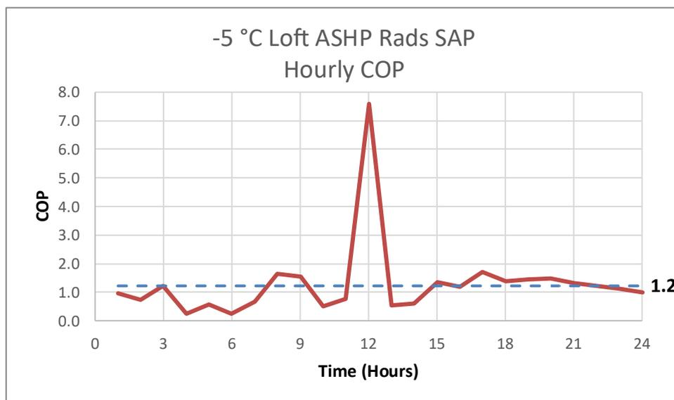
Figure 47. -5 °C Loft ASHP Rads SAP – Hourly COP
