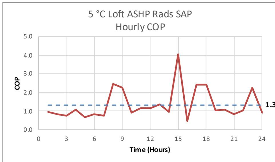
Figure 95. 5 °C Loft ASHP Rads SAP – Hourly COP
