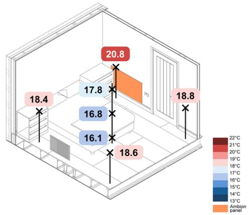
Figure 27. -5°C Wall Mounted IR TFH SAP - Spatial Operative Temperatures
