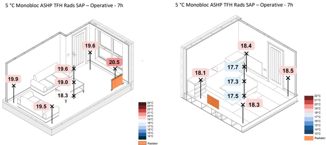
Figure 113. 5 °C Monobloc ASHP TFH Rads SAP – Spatial Operative Temperatures
