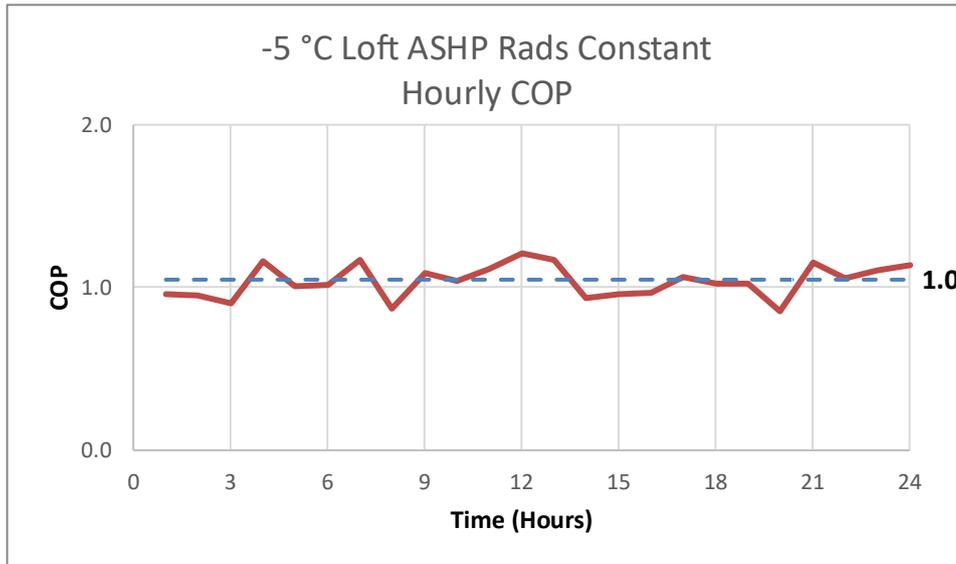
Figure 42. -5 °C Loft ASHP Rads Constant – Hourly COP
