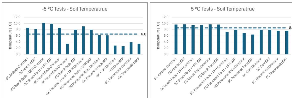
Figure 164. Soil Temperatures in -5 °C and 5 °C tests
