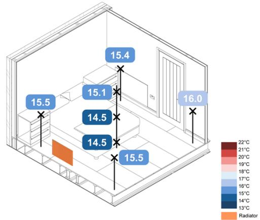
Figure 35. -5°C Loft ASHP Rads + UFH SAP – Spatial Air Temperatures
