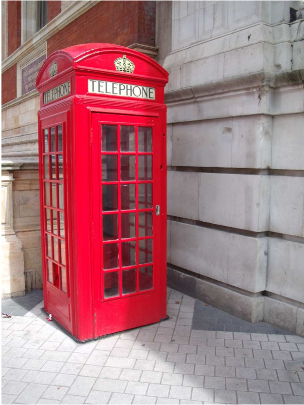
Figure 15. K2 kiosk outside the Victoria and Albert Museum, London, showing wartime bomb damage to the right of the top two rows of windows. This Grade II Listed kiosk (Listing No. 1265488) also has completely non-authentic gold painted crowns (photograph taken 21 August 2012).
