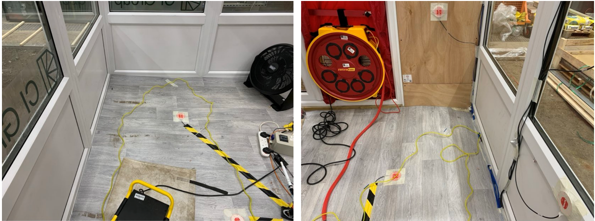
Figure 10 Disturbance to Floor Covering During Airtightness Testing
