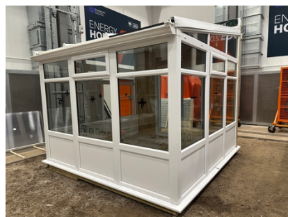
Figure 29 inside view of chamber 2 with the conservatory in-situ
