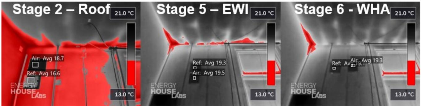
**Figure 29: Thermography of eaves and front and gable walls at test Stages 2, 5, and 6. Locations below the  $f_{CRsi}$  of 0.75 which are deemed to pose a risk of surface condensation and mould growth are highlighted in red (measurements on glazing panels are unreliable)**
