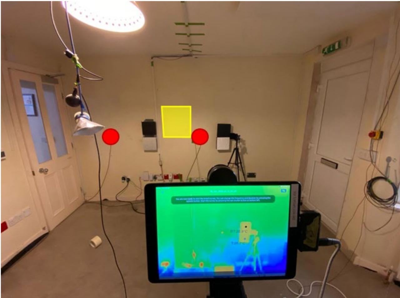
**Figure 7: Heat3D external wall U-value measurement. Yellow square denotes Heat3D measurement area and red circles the location of HFPs EW1 and EW2**
