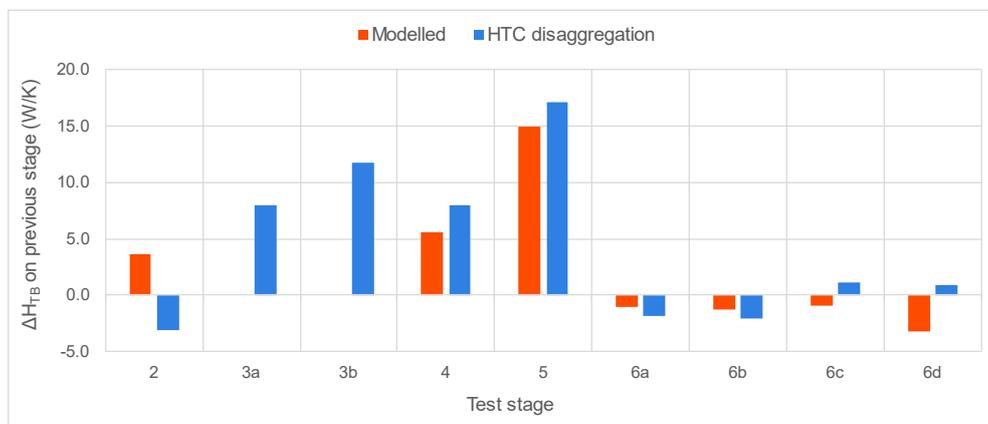
**Figure 25:  $H_{TB}$  change on previous test stage based on thermal modelling and HTC disaggregation (Stage 3b is change from Stage 2 and Stage 4 is change from Stage 3a)**
