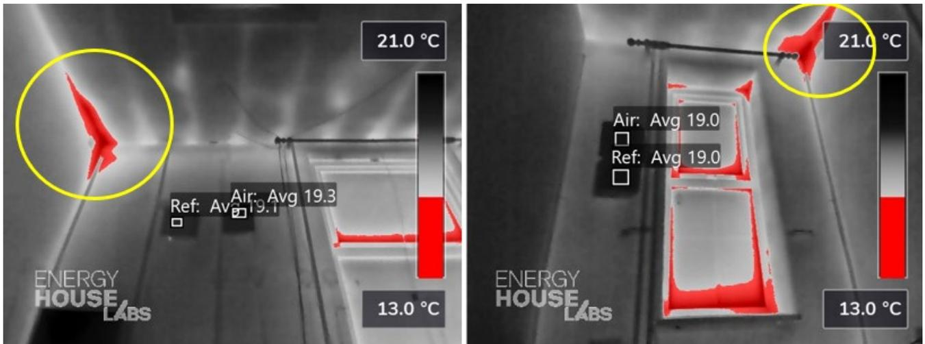
**Figure 31: Thermography of eaves/gable interface at verge (circled) on both the front (left) and rear (right) elevations after the whole house approach retrofit. Locations below the  $f_{CRsi}$  of 0.75 which are deemed to pose a risk of surface condensation and mould growth are highlighted in red (measurements on glazing panels are unreliable)**
