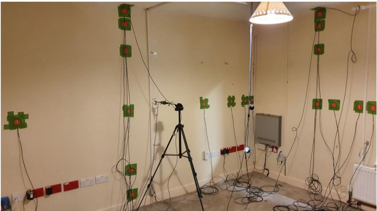
**Figure 6: HFPs on the external walls of bedroom 1 measuring heat flux density**
