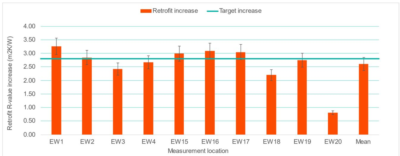
**Figure 18: External wall retrofit R-value increase at non-bridged locations**
