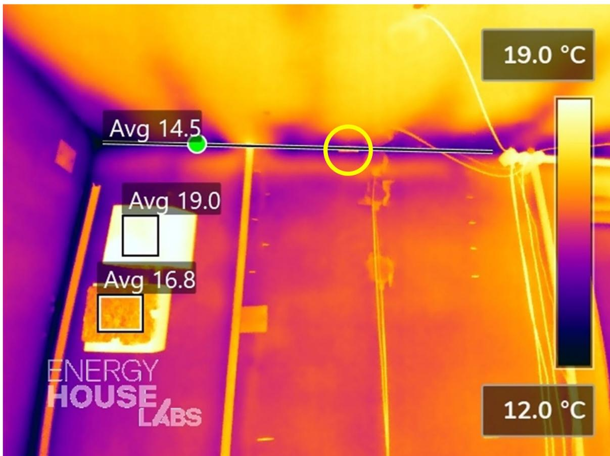
**Figure G1: Thermogram of the eaves junction in Bedroom 1 at Stage 2 of the DEEP retrofit. Location of surface temperature thermocouple circled**
