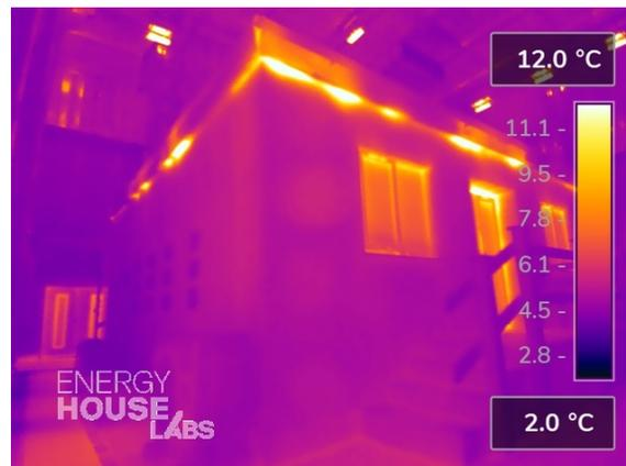
Figure 22. Exterior view of Vector V1 roof during pressurisation test
