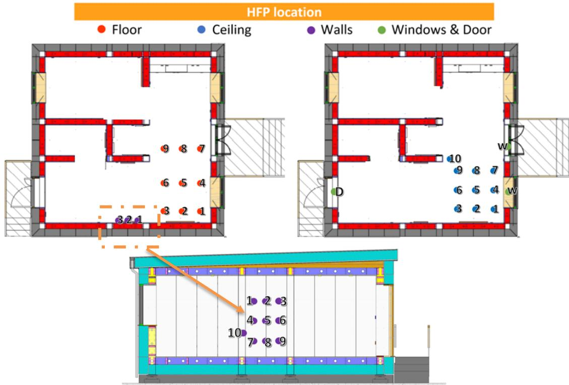
Figure 11. HFP locations on the external elements of Vector V1 (wall measurements were conducted on the right façade).
