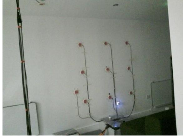
Figure 7. Heat flux measurements – wall
