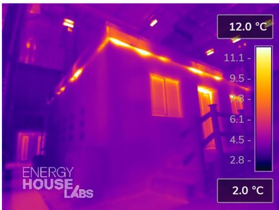
Figure 21. Exterior view of Vector V1 roof under no artificially induced pressure differential
