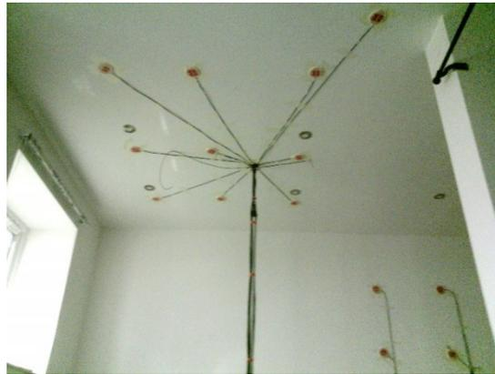
Figure 8. Heat flux measurements - ceiling
