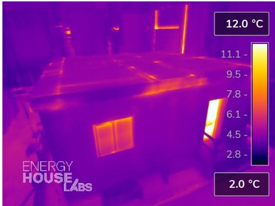
Figure 19. Exterior view of Vector V1 under no artificially induced pressure differential
