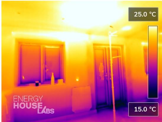
Figure 17. The french door under no artificially induced pressure differential
