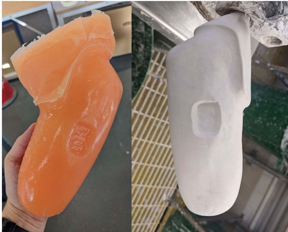
Figure 1. Left: Silicone negative mold produced from original socket; right: smoothed plaster negative mold produced from silicone negative via an alginate positive.
