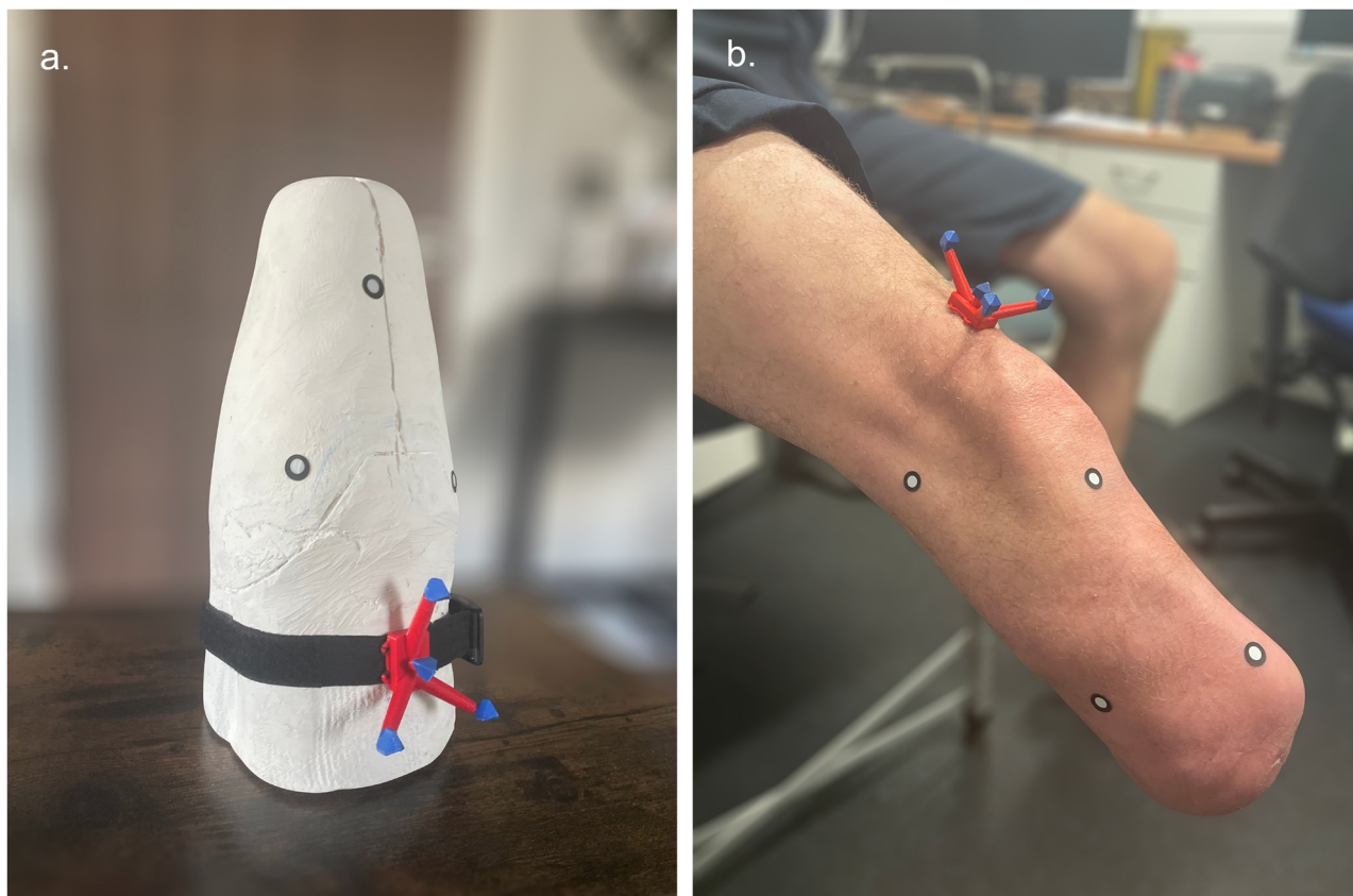
Fig 2. Scanning setup for transtibial model and limb. (a) Transtibial model used for evaluating the performance of each application between environments. (b) Transtibial limb of exemplar participant during scanning.
