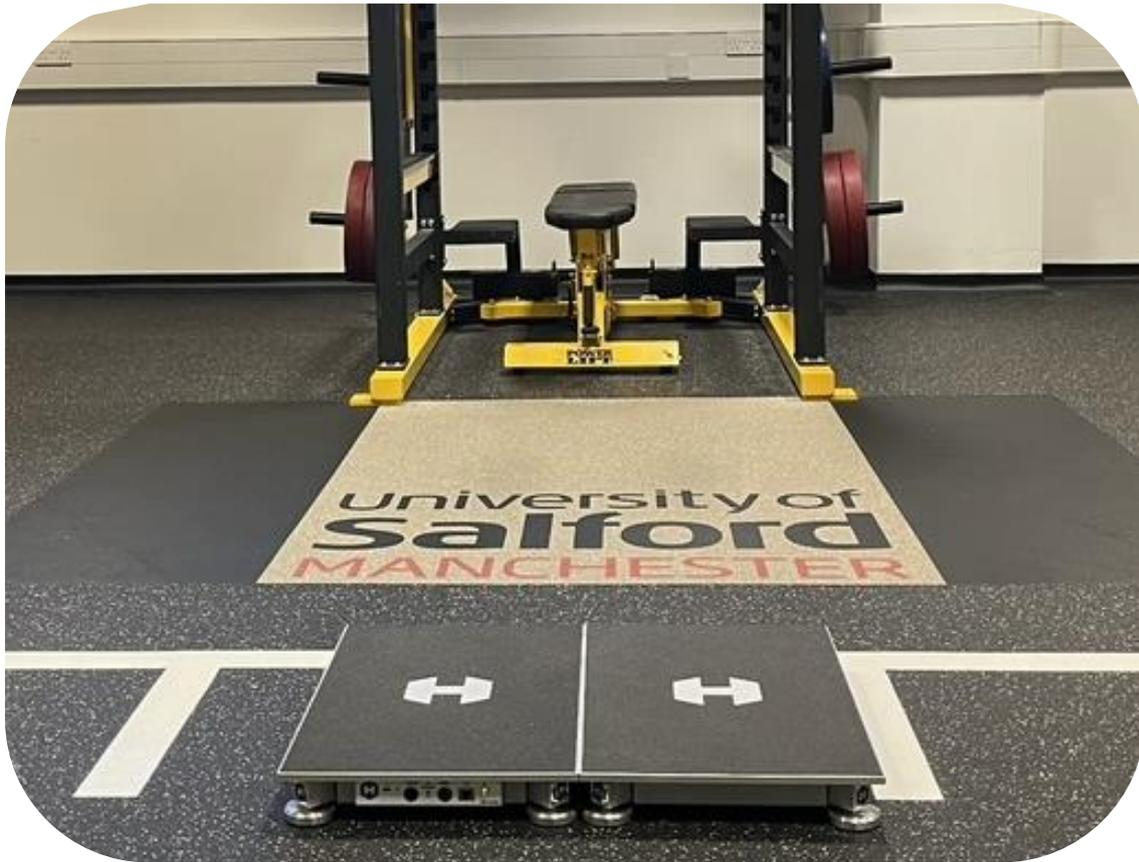
**Figure 5.1.** Example force plate system set-up without the foam surround.
