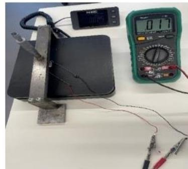
(b) Force being applied to the sensor
