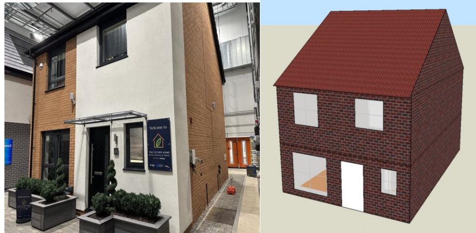
Figure 1. Front elevation of TFH in Energy House 2.0 environmental chamber one (left) and TFH modeled in DesignBuilder (right).
