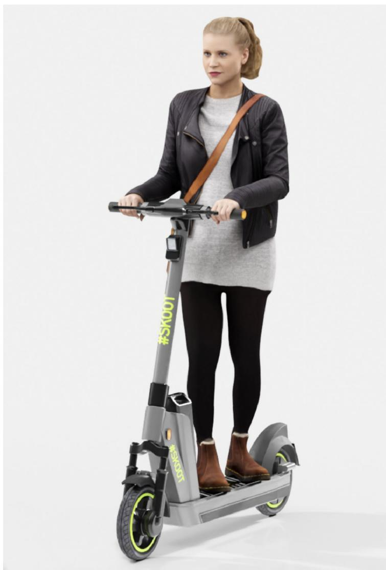
**Fig. 1.** Example of the computer generated e-scooter graphics used in the VR experiment. The models were generated with photogrammetry and included animation of both rider and e-scooter from motion capture data.
