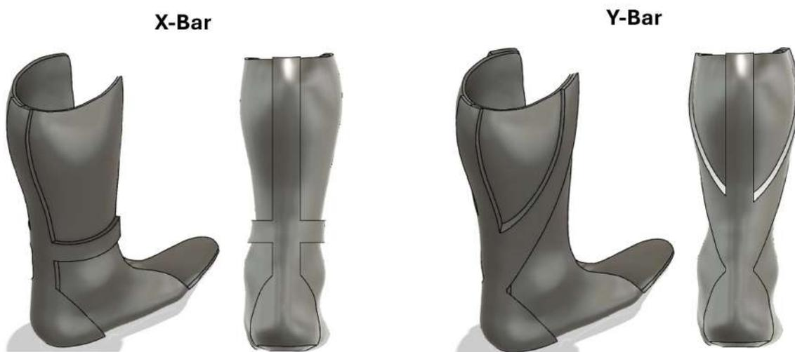
Figure 7.7: Proximal Reinforcement Design
