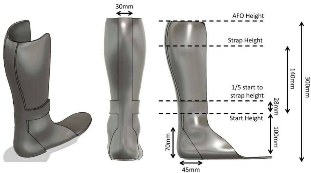
Figure 7.13: 10-year-old-sized AFO X-Bar Reinforcement Design
