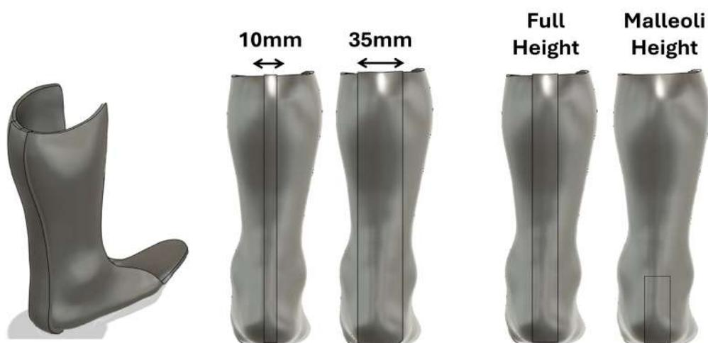
Figure 7.2: Rear Reinforcement Design
