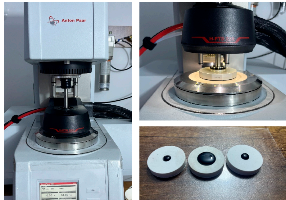
Figure 4. DSR-type SmartPave 102 e and testing specimens.
