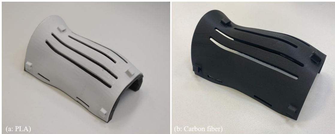
Figure 10-23: Fabricated anchor points. (a): PLA. (b): Carbon fiber.
