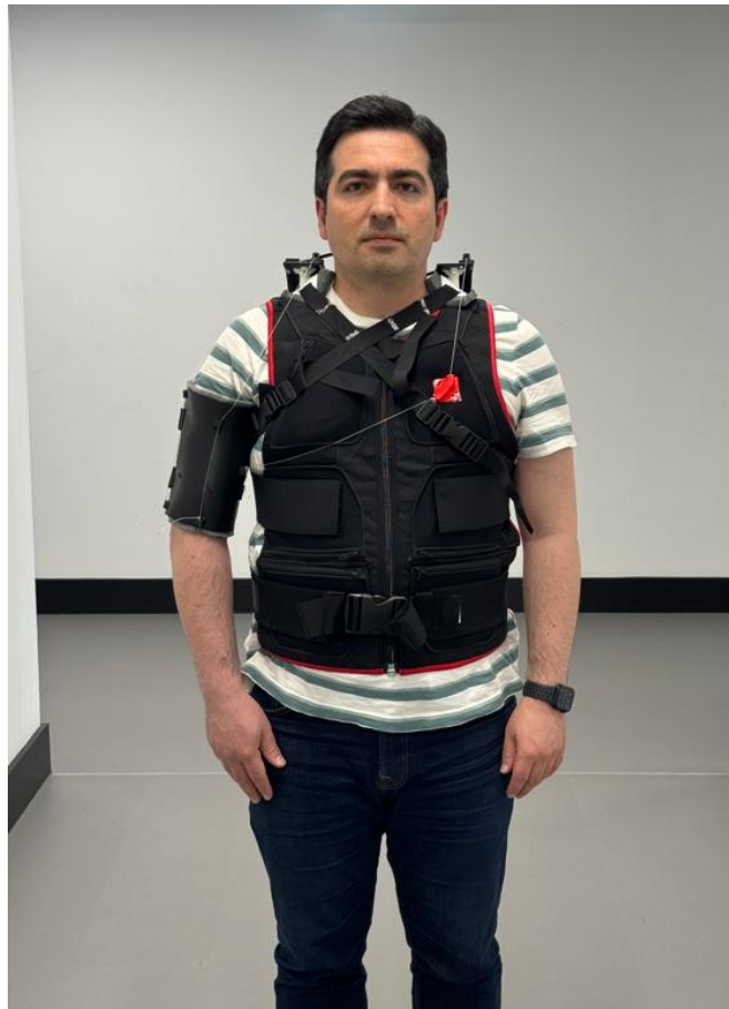
Figure 7-70: Carbon fiber CDSE worn by healthy candidate.
