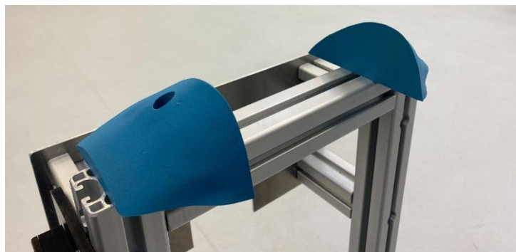
Figure 5-20: Installation of backpack seats on test bench.
