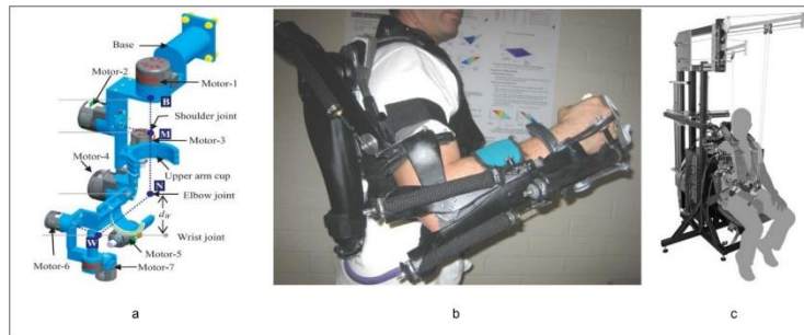
Figure 2-31: a: electric actuator [17]; b: pneumatic actuator [42]; c: hydraulic actuator [110].
