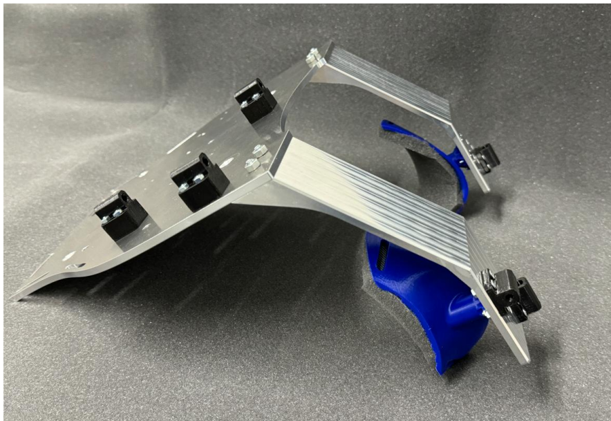
Figure 10-22: Positioning of Bowden cable housing on backpack (Type 1 and type 2).
