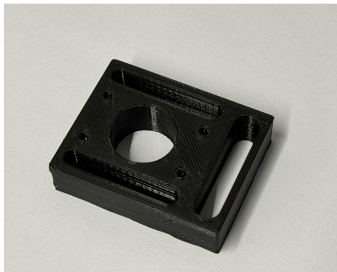
Figure 10-28: Fabricated motor mountain plate.
