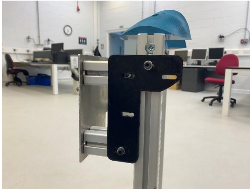
Figure 5-21: Installation of connection plate to the stand.
