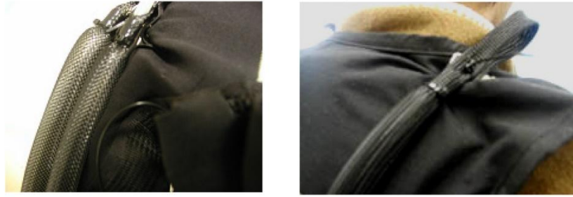
Figure 2-34: Sample of slippage and wear when operating a pneumatic actuator[36].
