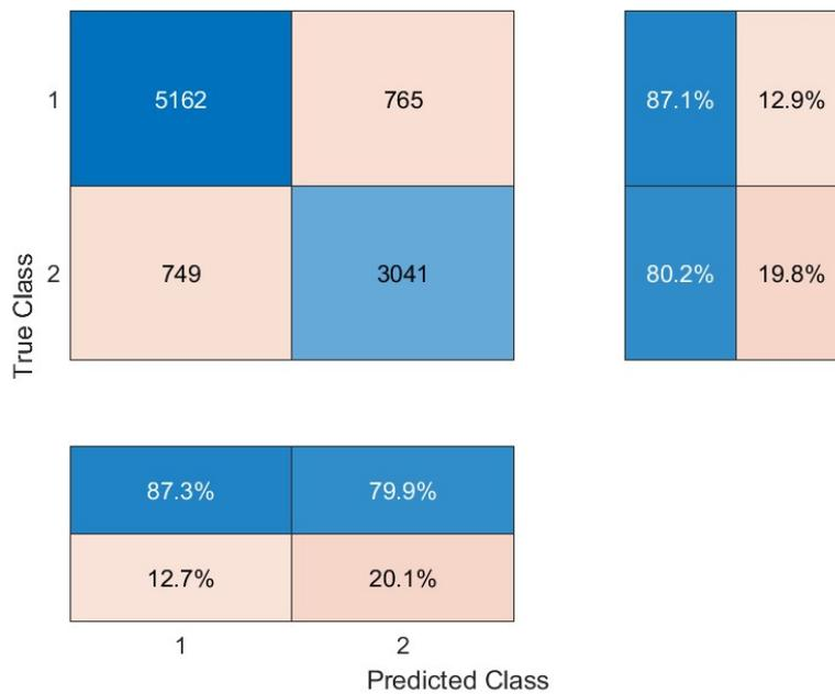
Fig. 7.2 Confusion matrix for walking aid recognition Cross-validation SVM optimised trial. 1-without a walking aid 2-with a walking aid
