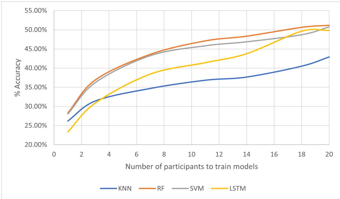
Fig. 4.23 Average percentage accuracy against the number of participants used to train the classification models. One to twenty participants were used to train four machine learning models: K-Nearest Neighbors (KNN), Long Short-Term Memory (LSTM), Random Forest (RF), and Support Vector Machines (SVM). Using more participants to train the models produced higher average percentage accuracies for all models.
