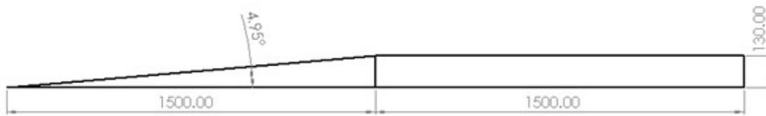
Fig. 5.2 Ramp set up as used for data collection in the gait lab. Lengths in mm.
