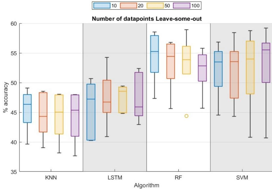
Fig. 4.13 Leave-some-out accuracy results for terrain classification across different number of datapoints per window. The boxplot shows the classification accuracy for each number of datapoints (10, 20, 50, 100) using four machine learning algorithms: K-Nearest Neighbors (KNN), Long Short-Term Memory (LSTM), Random Forest (RF), and Support Vector Machines (SVM). The number of datapoints didn't affect the accuracies using all algorithms.
