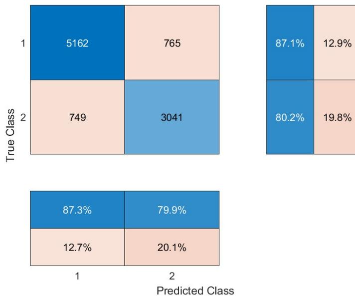
Fig. 4.48 Confusion matrix for walking aid recognition cross-validation SVM optimised trial. 1-withouth a walking aid 2-with a walking aid..
