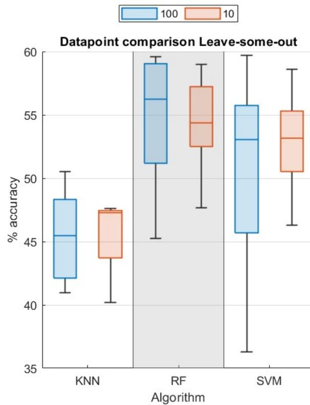
Fig. 4.24 Leave-some-out accuracy results for terrain classification across trials 10 and 100 datapoints. The boxplot shows the classification accuracy for 10 and 100 datapoints using the three best performing machine learning algorithms from the previous analysis: K-Nearest Neighbors (KNN), Random Forest (RF), and Support Vector Machines (SVM). Using 10 datapoints was not significantly different to 100 datapoints.
