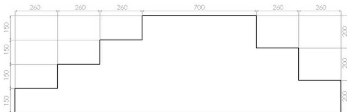
Fig. 5.1 Set of stairs used for data collection in the gait lab. Lengths in mm.
