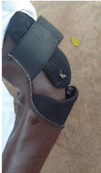
Fig. 7. Example of failure of a rivet.
