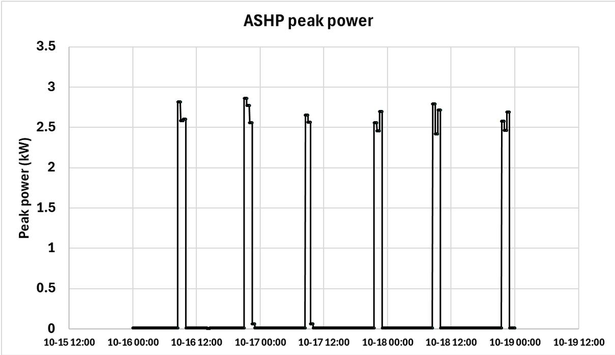
Figure 17. ASHP peak power during the 72-hour pre-test
