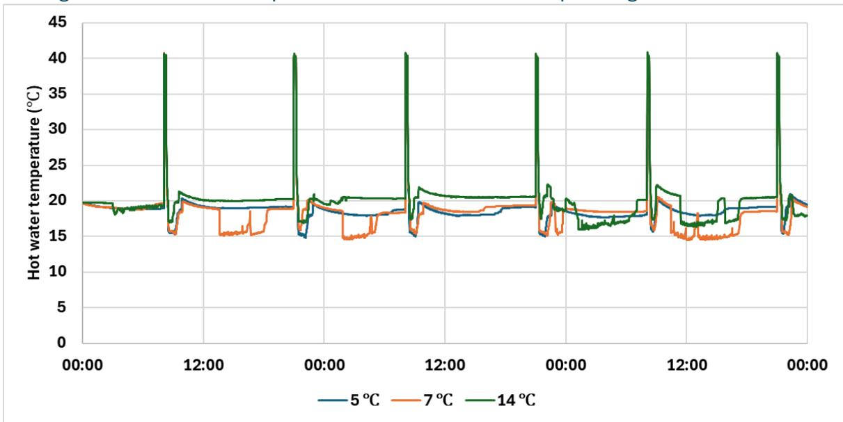
Figure 26 Hot water temperature of the bath tap during the 72-hour tests
