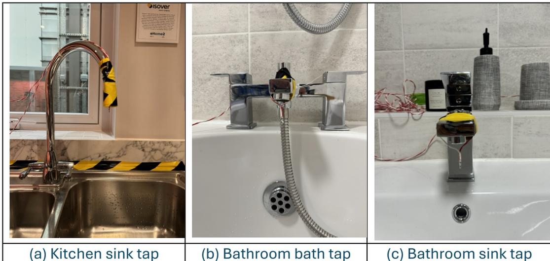
Figure 6 Type-T thermocouple sensors installed at tap outlet
