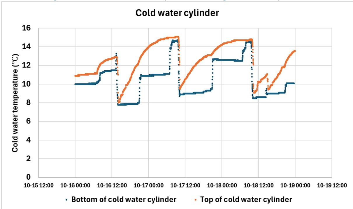
Figure 14. Cold water cylinder temperature during the 72-hour pre-test
