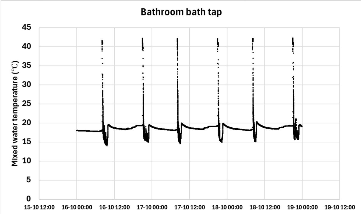
Figure 12. Bathroom bath tap temperature during the 72-hour pre-test
