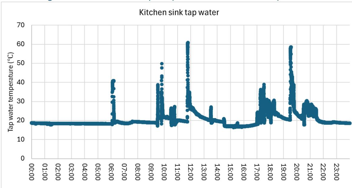
Figure 9. Kitchen sink tap water temperature during the 24-hour pre-test
