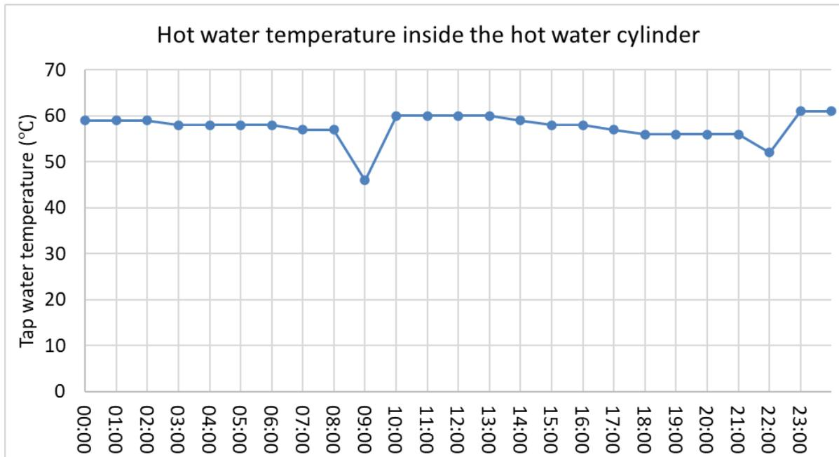
Figure 10. Hot water temperature inside the hot water cylinder during the 24-hour pre-test
