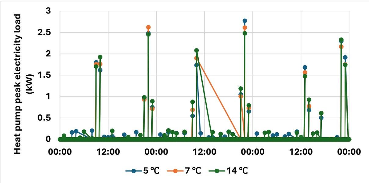
Figure 24. Heat pump peak electricity load during the 72-hour tests
