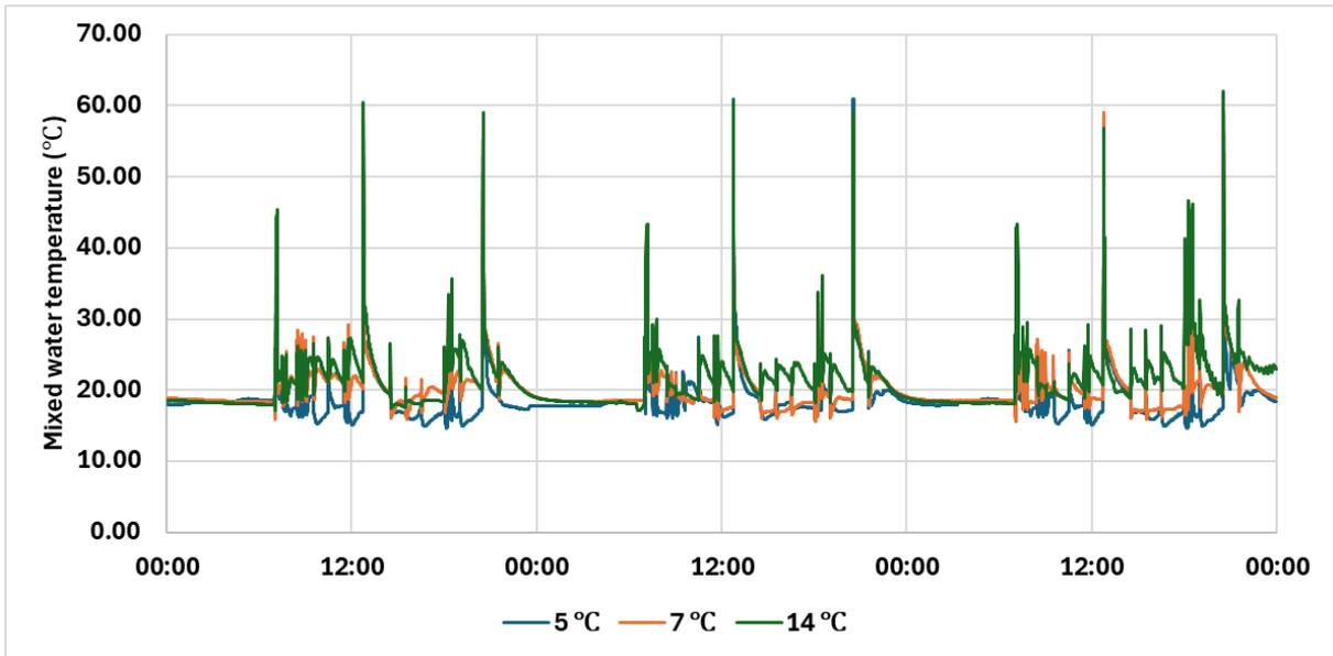
Figure 19. Mixed water temperature of the Kitchen sink tap during the 72-hour tests
