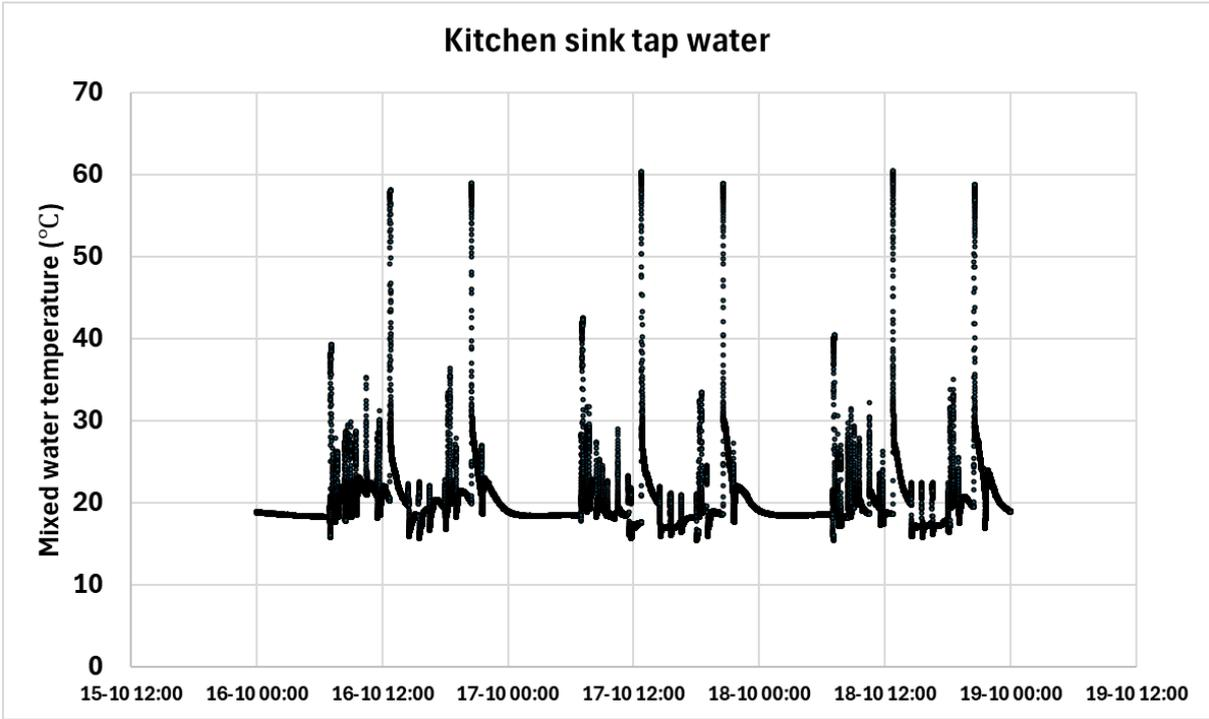
Figure 11. Kitchen sink tap water temperature during the 72-hour pre-test
