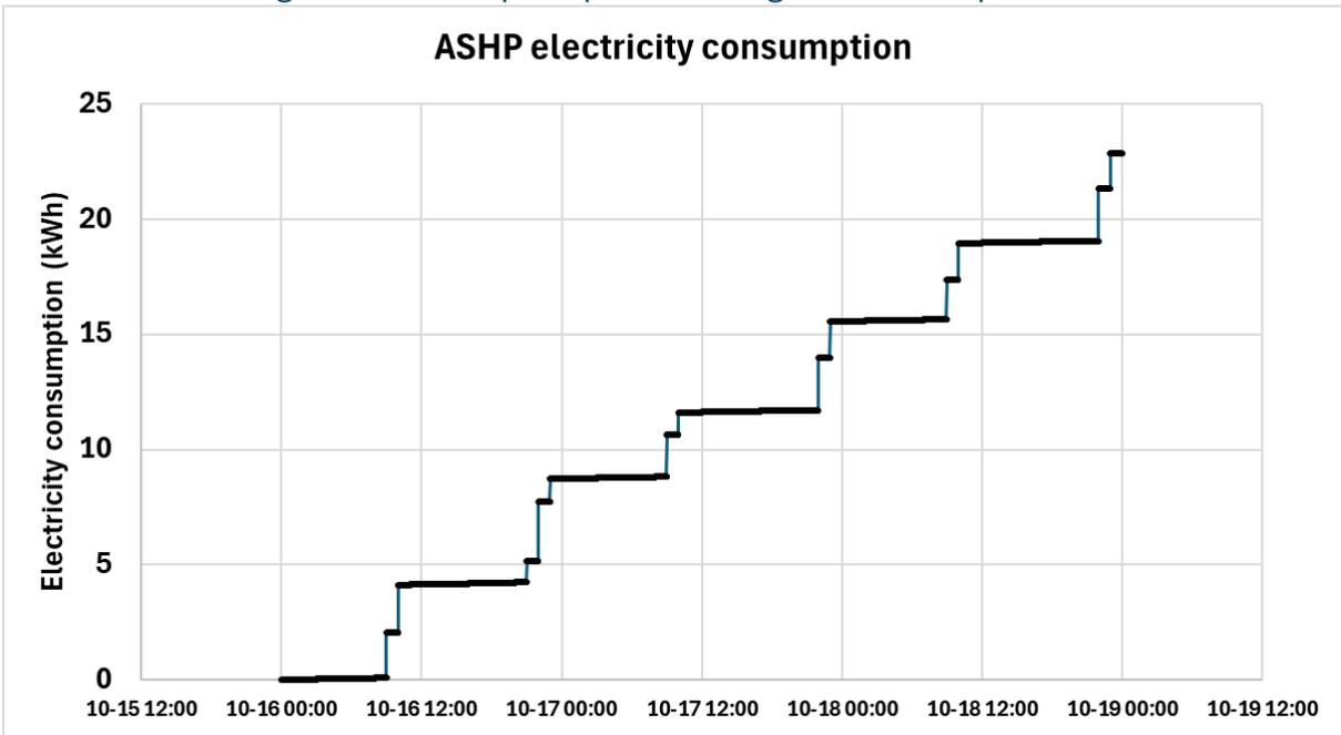
Figure 18. ASHP electricity consumption during the 72-hour pre-test
