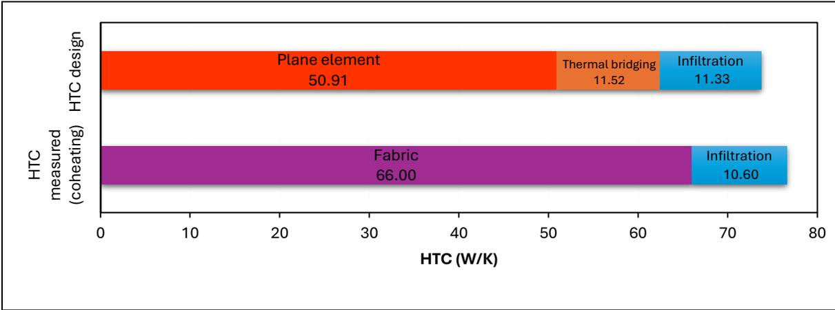
Figure 1. eHome2 HTC design vs measured (Fitton et al., 2024).
