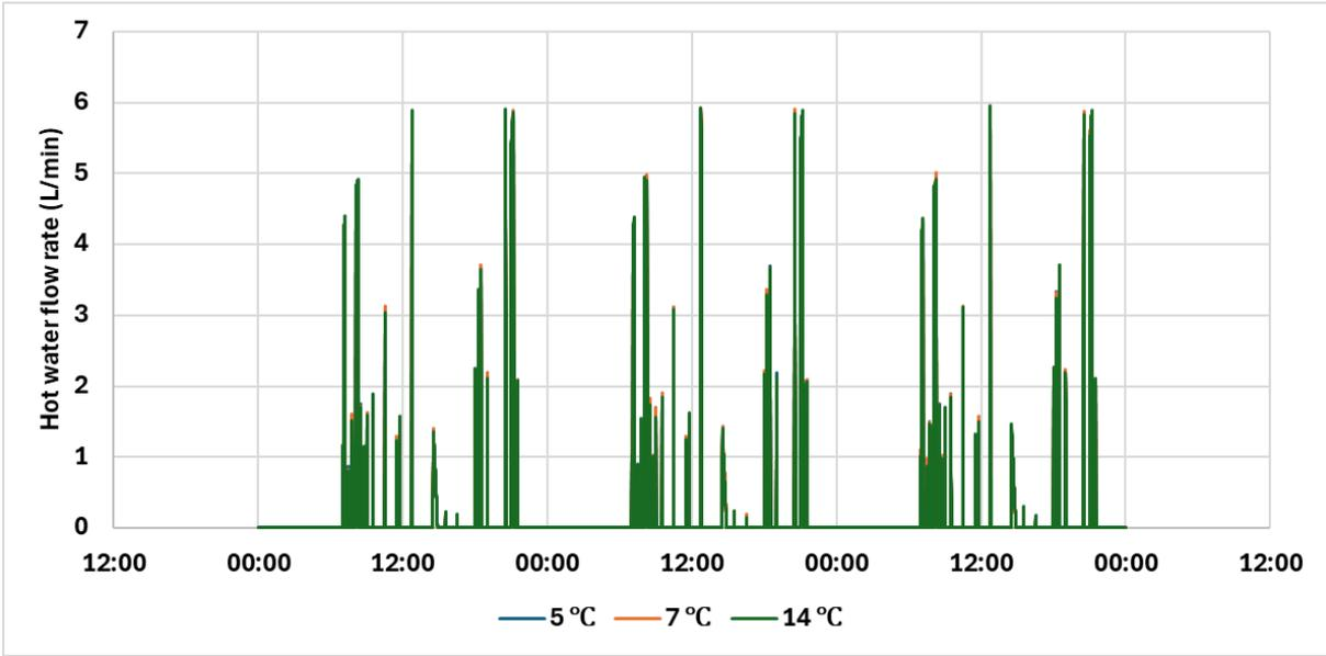
Figure 21. Hot water flow rate during the 72-hour tests
