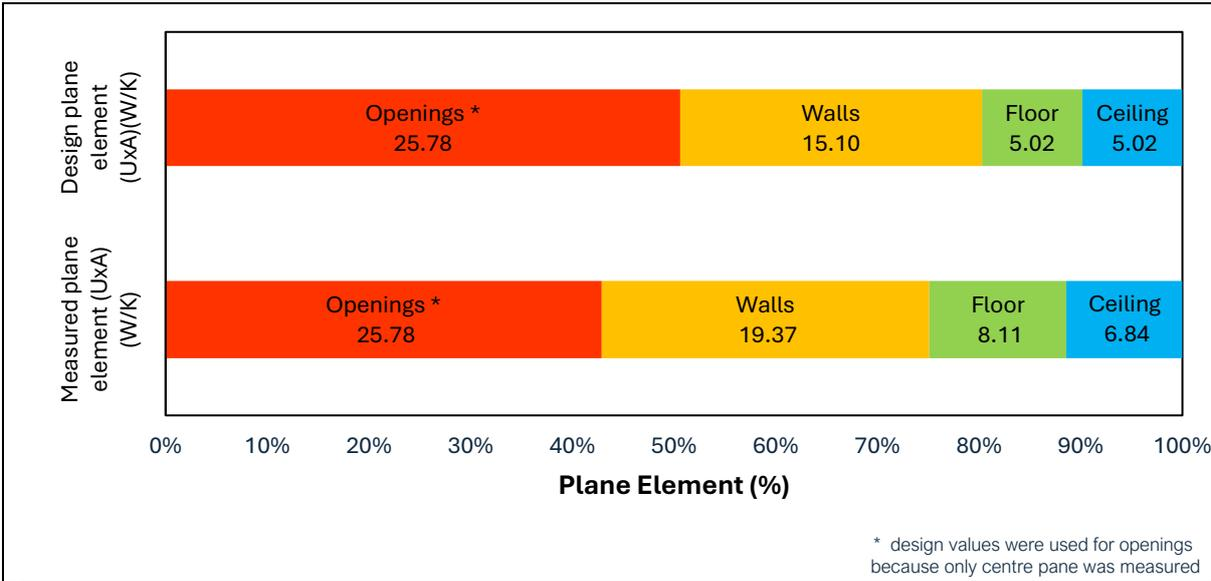
Figure 2. eHome2 Fabric Heat Loss by components (Fitton et al., 2024).
