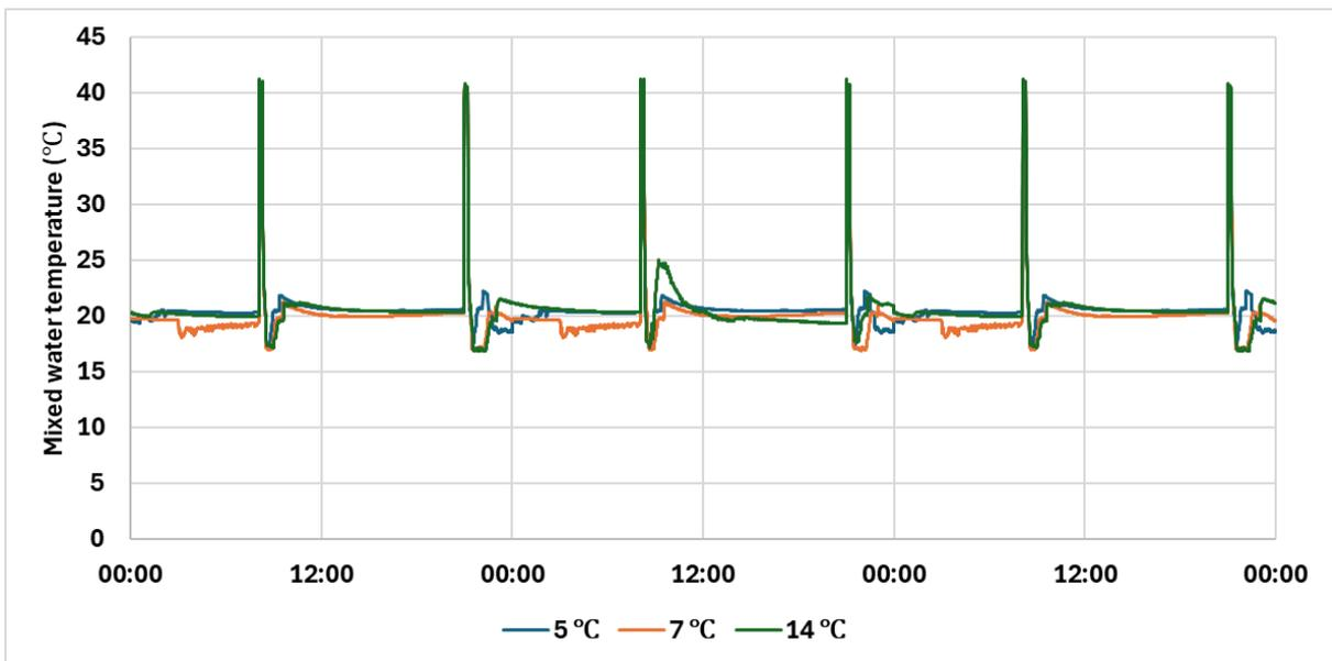
Figure 20. Mixed water temperature of the bath tap during the 72-hour tests
