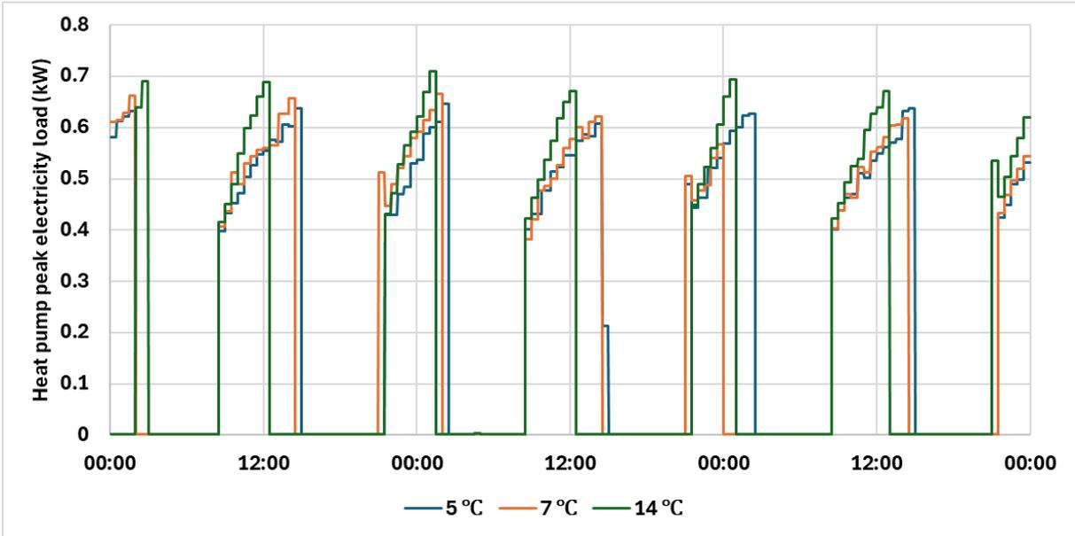
Figure 29 Heat pump peak electricity load during the 72-hour tests
