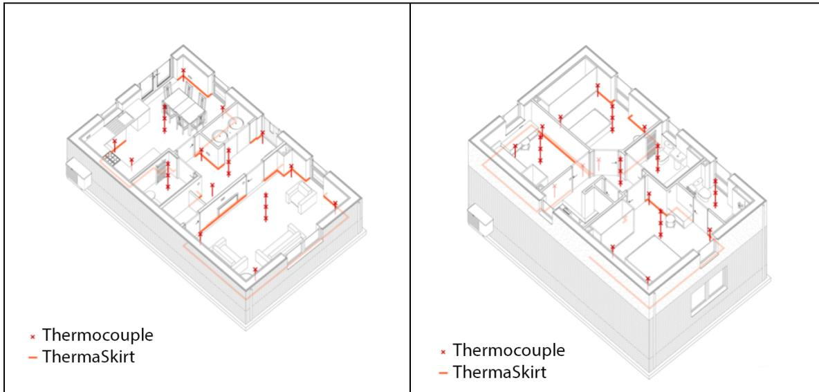
Figure 5. Heating emitters and sensors in eHome2 downstairs (left) and upstairs (right)
