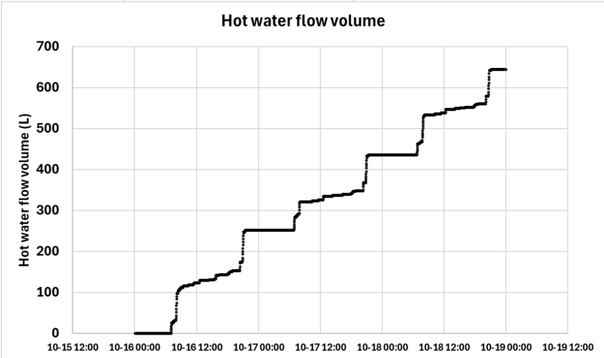
Figure 16. Hot water flow volume during the 72-hour pre-test
