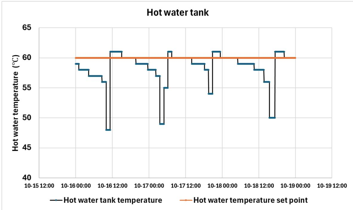
Figure 13. Hot water tank temperature during the 72-hour pre-test
