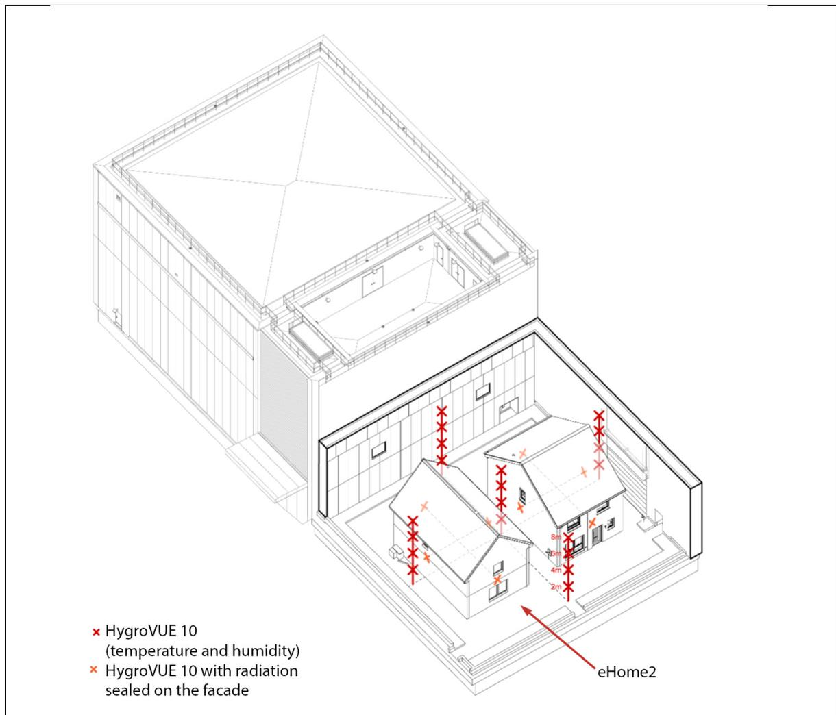
Figure 4. Diagram of air temperature and humidity sensor locations within the chambers
