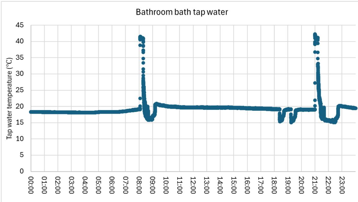
Figure 8. Bathroom bath tap temperature within a 24-hour pre-test
