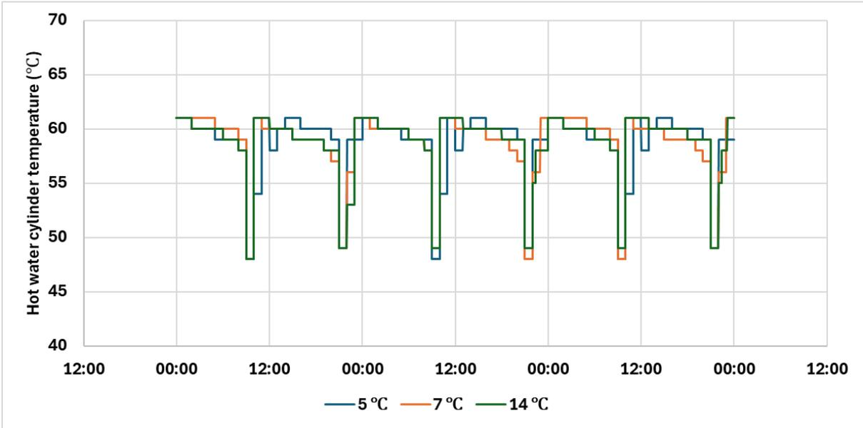
Figure 23. Hot water cylinder temperatures during 72-hour tests
