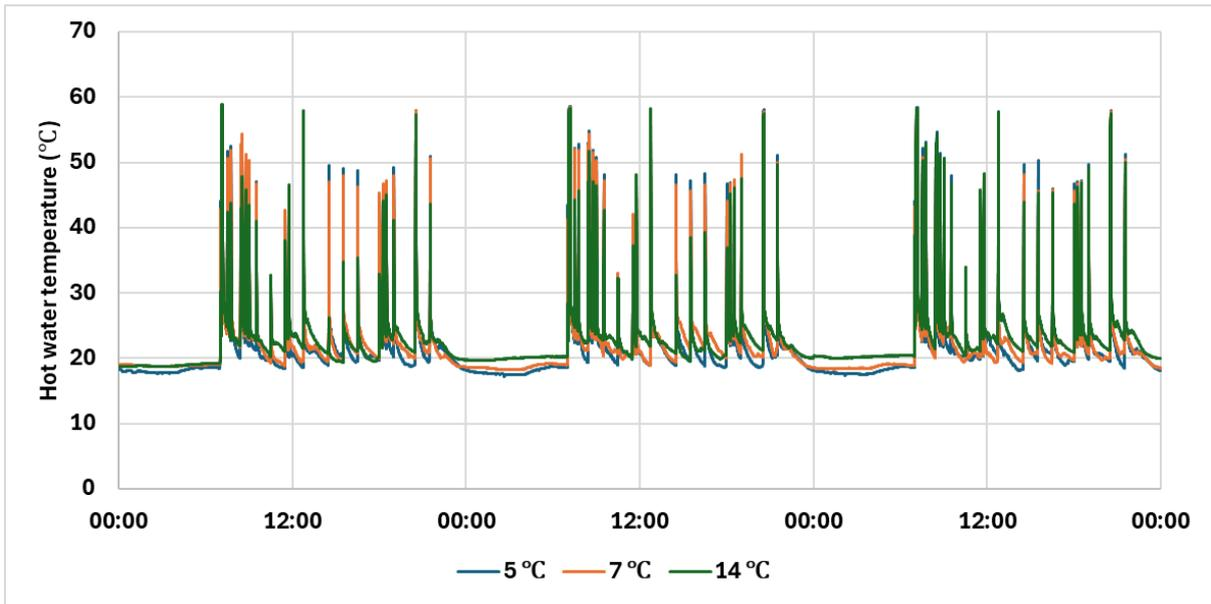
Figure 25 Hot water temperature of the Kitchen sink tap during the 72-hour tests
