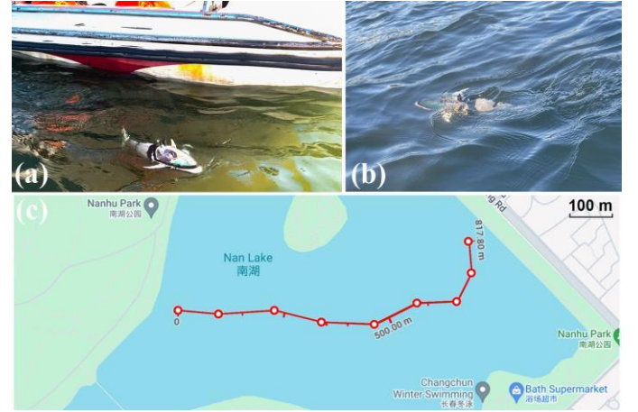
Fig. 16. Swimming test in open water. (a)(b) Photo captured from boat. (c) Approximate trajectory of HyperTuna.
