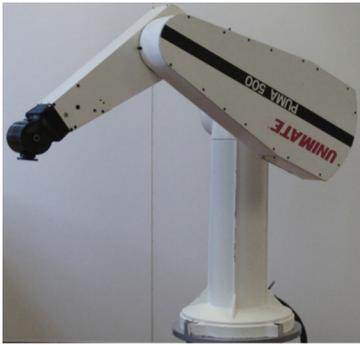
**Fig. 2** The Puma 560 robot manipulator
