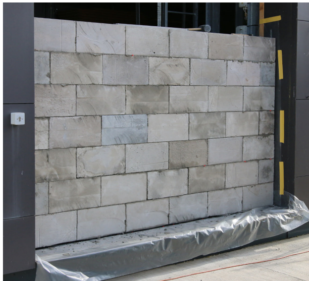
Figure 8: Masonry wall assembled from industrially produced lightweight blocks for long-term monitoring of thermal and hygric properties.
