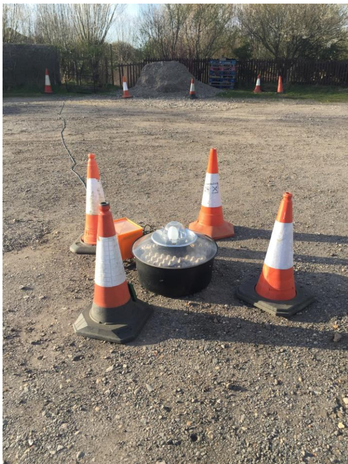
Figure 2: The Robinson Moth-Trap set-up for deployment in the Observatory car park, note the Pyrex Bowl over the bulb to prevent shattering due to water contact (Gregory Lee).
