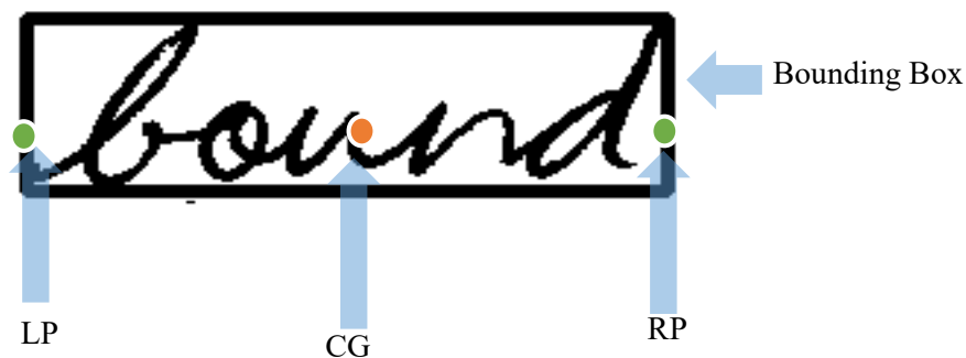
Fig. 11. Examples of the Left-most Point (LP) boundary, Center of Gravity (CG), and Right-most Point (RP) boundary in a component.
