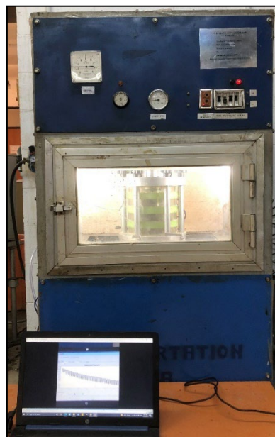
Figure 5. Triaxial test for resilient modulus.
