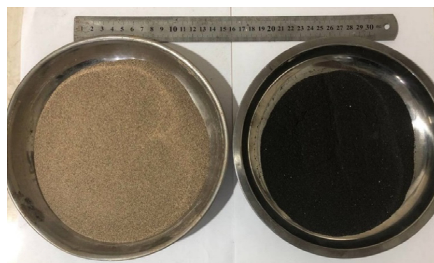
Figure 2. The iron filings and FNS.
