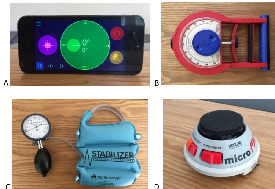
Figure 3.2 – Measurement instruments: a) Goniometer Pro app; b) handgrip dynamometer; c) pressure biofeedback; d) hand-held dynamometer.
