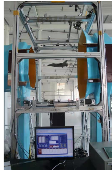
Figure 16. A flat moving platform inside the aircraft in the wind tunnel test.
