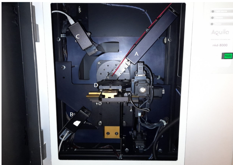
Figure 11. Image of the Aquila NKD-8000 used in this study. A) beam tube, B) Transmittance detector, C) Reflectance detector and D) Sample stage. UV-Vis has been routinely used for the characterisation of MAPI exhibiting an absorption edge occurring at approximately 770 nm.
