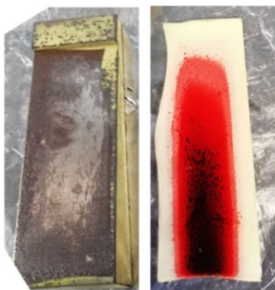
Figure 25. Sample S6 removed from furnace early as solution had depleted. Distinct regions of varying stages of formation are observable with black being perovskite and off-white being PbI_2 . Red region still unidentified. Approx dimensions = 7cm x 2cm.
