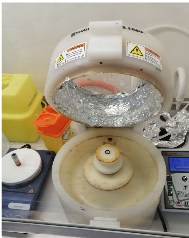
Figure 8. Illustrating a spin-coater.
