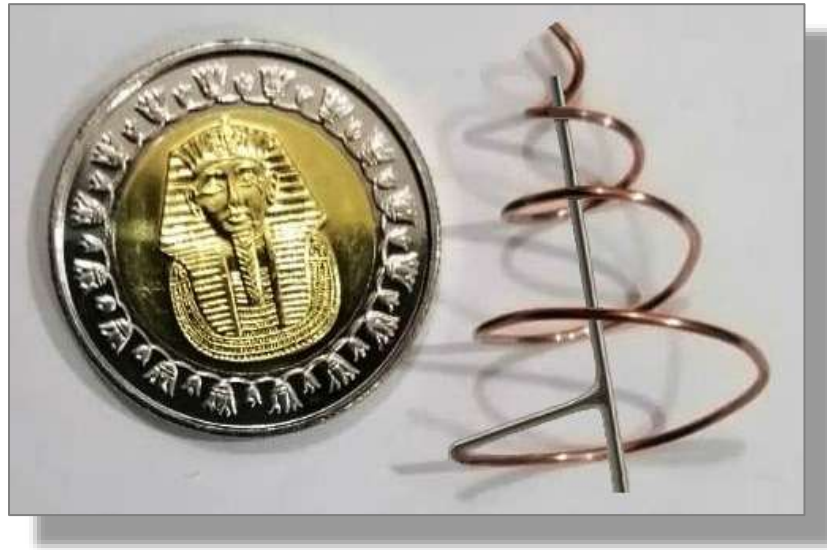
Figure 6.5: A copper wire is wrapped to form a conical helix and then welded to a straight wire to form the conical-helix/monopole antenna proposed to play the role of a central on-body antenna for on-body biosensor antenna network
