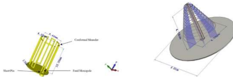
Figure 2.15: (a) Simulated Meander Antenna for Capsule Endoscopy. (b) Spiral Helix Antenna for outside application. [97]
