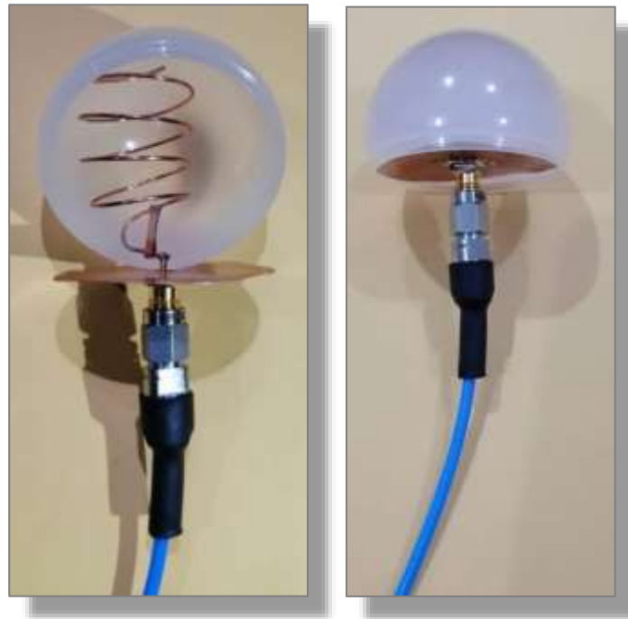
Figure 4.28: The matched cylindrical helix antenna on a copper circular disc with SMA connector is being covered with hemispherical radome.
