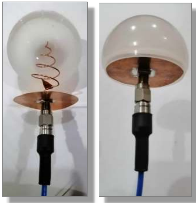
Figure 4.30: The matched conical helix antenna on a copper circular disc with SMA connector is being covered with hemispherical radome.
