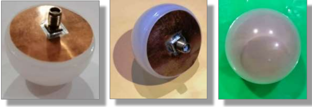
Figure 4.27: The fabricated prototypes of the three proposed helical antennas mounted on a circular copper disc and covered by hemispherical radome with SMA feeding connector.
