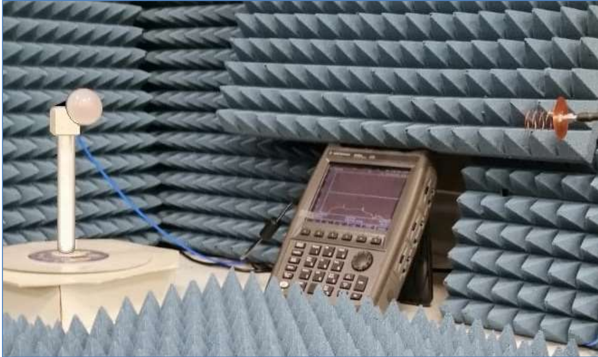
Figure 4.38: Experimental setup for measuring the radiation pattern of the proposed on-body helical antennas using the VNA of the Agilent Field Fox N9918A.
