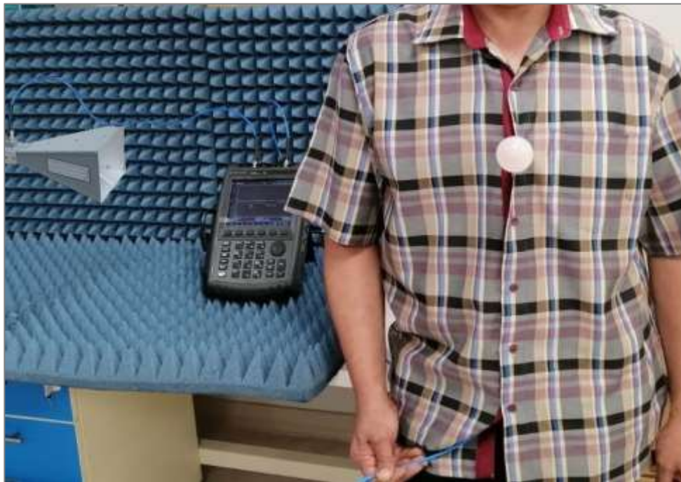
Figure 6.13: Experimental setup for measuring the radiation patterns of the conical-helix/monopole antenna on the human body using the VNA of the Agilent Field Fox N9918A.
