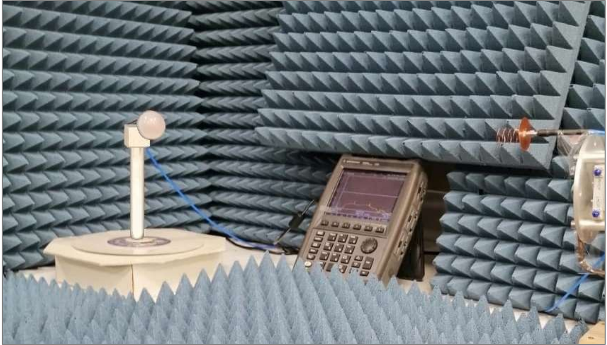
Figure 6.12: Experimental setup for measuring the radiation pattern of the proposed on-body conical-helix monopole antenna in free space using the VNA of the Agilent Field Fox N9918A.
