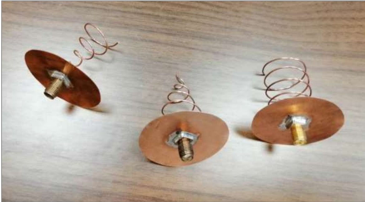
Figure 4.23: The fabricated prototypes of the three proposed helical antennas mounted on a circular copper disc with SMA connector for feeding (without being covered by the radome).
