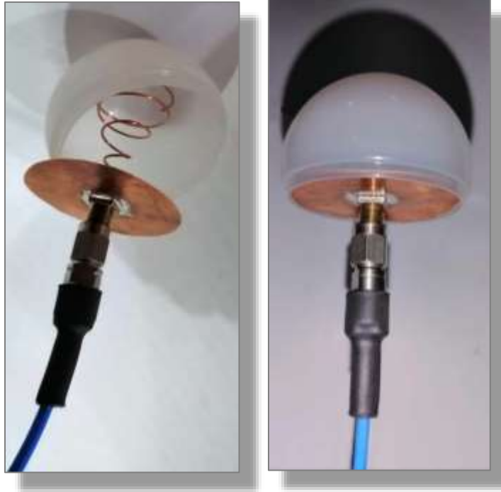
Figure 4.29: The matched inverted conical helix antenna on a copper circular disc with SMA connector is being covered with hemispherical radome.
