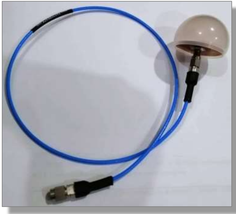
Figure 4.31: The final form of the proposed on-body medical antenna connected to a coaxial cable for the purpose of experimental measurements.
