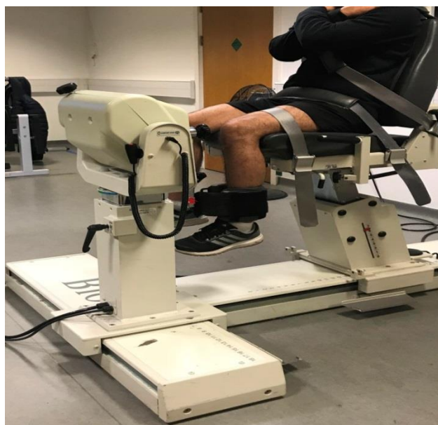
Figure 3-14 Participant position for MVIC test of the hip external rotators
