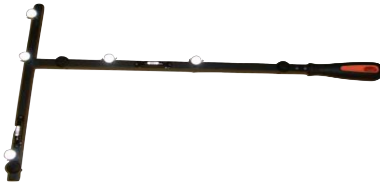
Figure 3-3 T-shaped calibration wand for the Vicon system
