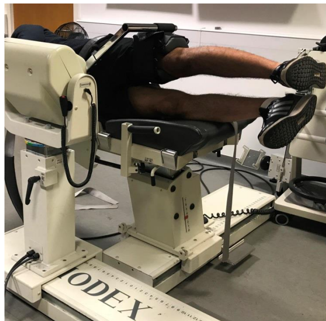
Figure 3-12 Participant position for MVIC test of the hip abductors
