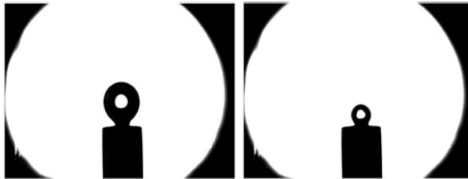
Fig. 9. Bubble shrinkage of CO 2 bubble in Distilled water I: Onset R: End (10 s interval).
