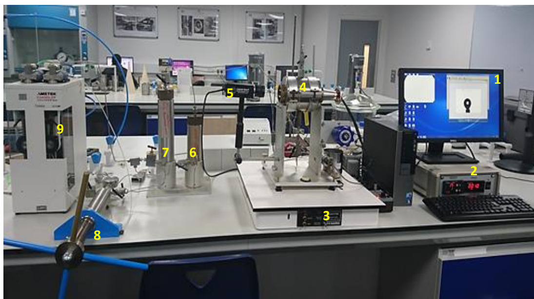
Figure 3.21 Experimental setup for ST measurement (1 Computer, 2 Temperature and pressure controller, 3 Vibration control bench, 4 ST cell, 5 Rame-hart camera, 6 &7 Accumulators, 8 manual pump, 9 Automatic pump)
