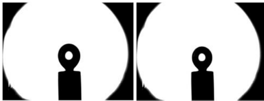
Fig. 11. Bubble shrinkage of CO 2 in 10 wt% brine L: Onset R: End (10 s interval).
