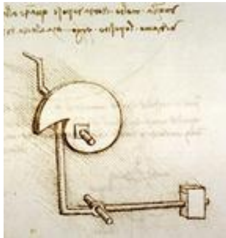
Leonardo Da Vinci, Mechanical hammer with eccentric cam
