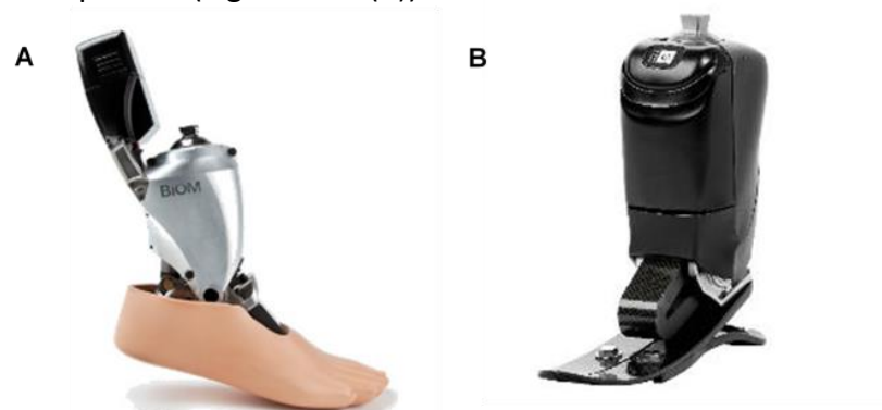
Figure 2.30 (A) The BiOM foot in an earlier version (figure sourced from Mancinelli et al. (2011)). (B) Version currently commercialised by Ottobock with the name of "Empower" (image sourced from shop.ottobock.us ).
