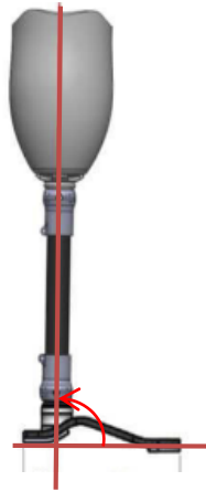
Figure 2.3 Example of the neutral angle for a prosthetic foot, defined as the angle between the prosthetic foot and the prosthetic shank during standing position. Figure adapted from Medical EXPO (2018).
