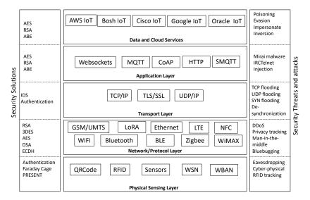
**Figure 1.** The proposed IoT architecture.
