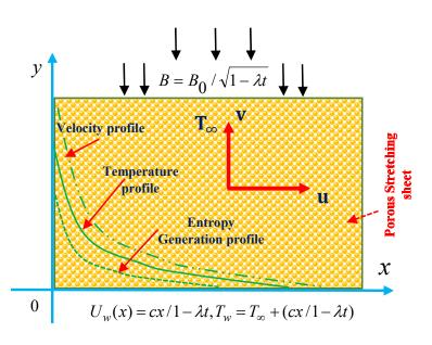
Fig. 1. Schematic of the physical model
