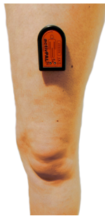
Figure 5.1: Placement of the activPAL3C device on the thigh.
