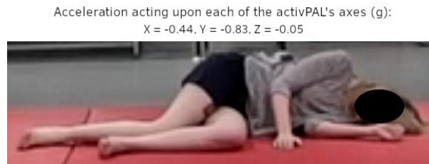
Figure 5.9: Lying on the left side post-fall. The incline of the thigh with respect to the floor results in a lower acceleration due to gravity on the activPAL's Y-axis compared to if the thigh had been parallel to the floor. Despite the participant being fully rotated onto their left side, the acceleration due to gravity on the activPAL's Y-axis is less than the threshold devised by Lyden et al. [171] ( Y > 0.906 ) and so lying was not detected when their threshold was used.
