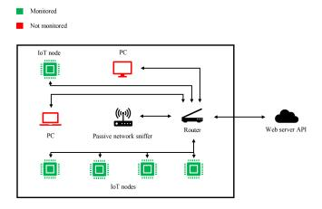
Fig. 2. AWPA-2 Protected WLAN and sniffer setup.
