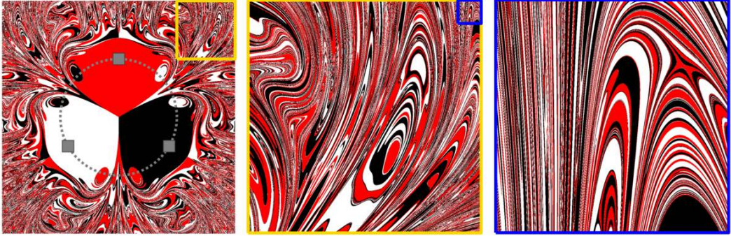
Figure 1. Basins of attraction for the magnetic pendulum with b = 0.1 and h^2 = 1/4 . In the first pane, the grey squares denote the position of the base-plane magnets and the dotted grey line is a circle with radius equal to the unit length. The second and third panes show successive magnifications.
